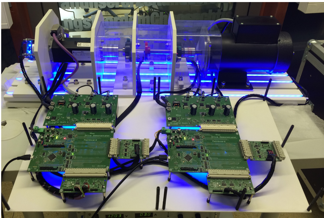
Figure 5.6: Mechanical Setup - the mechanical construction of the Dunkermotor and the Ohio Electric motor
