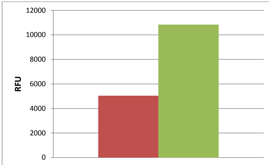
Figure 46. Relative fluorescing unit measurement of R. eutropha H16 [pKRSF1010_Ptac_eGFP] (red) and R. eutropha H16 ΩKmT7pol [pCM_PT7_RS F1010_eGFP_Pemlk_ΔlacI] (green). The difference of the eGFP expression under the regulation of P_{tac} and P_{T7} could be emphasized with the relative fluorescing unit measurement.
