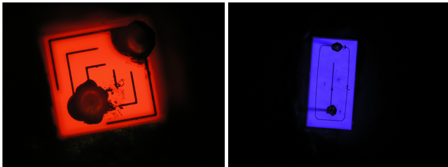
Figure 4.2.: Optical microscope images of the operated red emitting AlGaInP-based LED (left panel, image magnification 200 times) and the GaN-based LED (right panel, image magnification 50 times). The DC current level was 2 \mu\text{A} for the red emitting AlGaInP-based and 5 \mu\text{A} for the blue emitting GaN-based, respectively.
