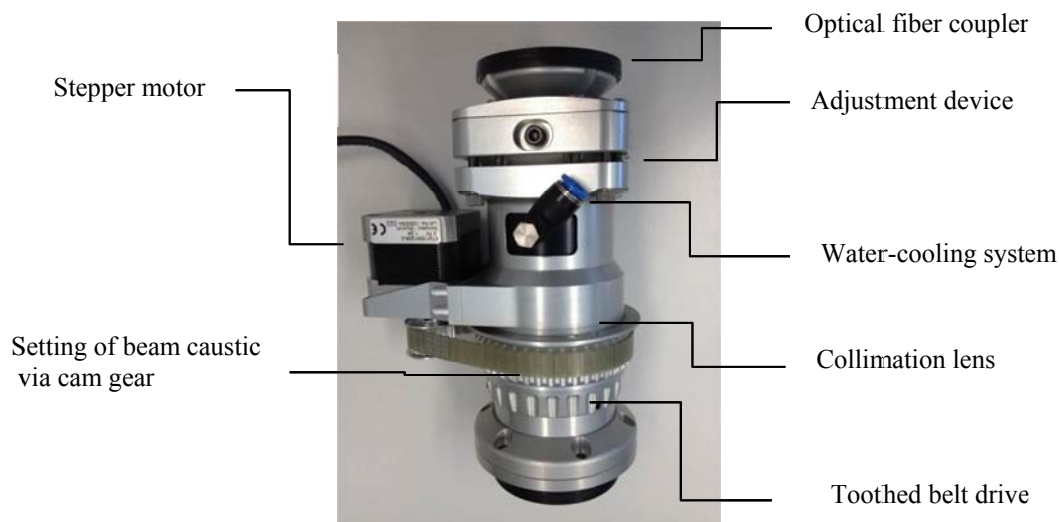
Figure 2-8: (a) Collimation unit and (b) geometry of applied collimation lens [67].
