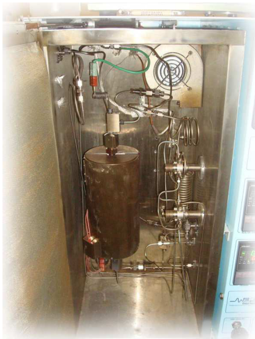
Figure 2: Interior of MICROACTIVITY-Reference – the hot box.
