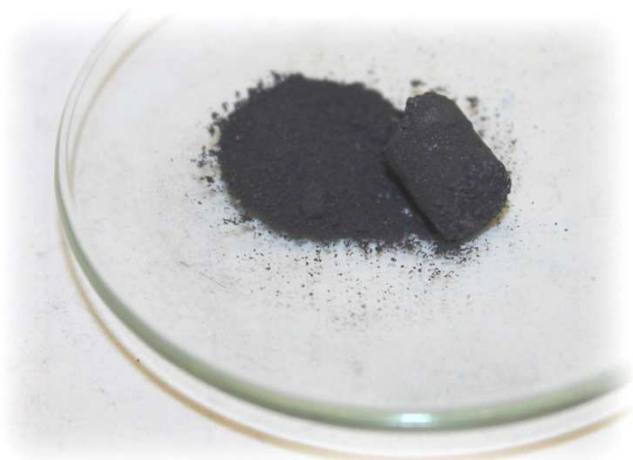
Figure 32: Sintered piece of contact mass. Reactivity immensely decreased by formation of such tight blocks.
