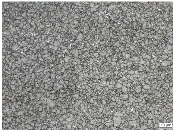
Abbildung C 104: WEZ Simulation (S 700MC, Blechdicke 10 mm), T_{\max}(1) = 962,2^{\circ}\text{C} , t_{8/5}(1) = 6,5 s, T_{\max}(2) = 954,5^{\circ}\text{C} , t_{8/5}(2) = 6,3 s
