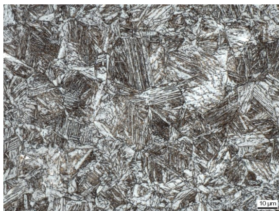
Abbildung C 106: WEZ Simulation (S 700MC, Blechdicke 10 mm), T_{\max}(1) = 729,4^{\circ}\text{C} , t_{8/5}(1) = 5,0 s, T_{\max}(2) = 1234,8^{\circ}\text{C} , t_{8/5}(2) = 6,1 s
