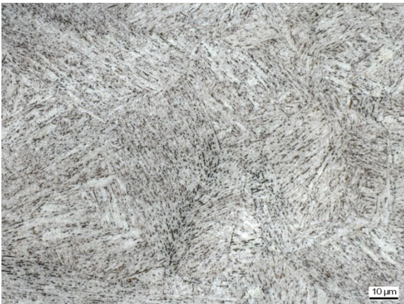
Abbildung 5-81: WEZ-Simulation (S 700MC, Blechdicke 10 mm), T_{\max}(1) = 1238,2 \text{ °C} , t_{8/5}(1) = 5,1 \text{ s} , T_{\max}(2) = 720,6 \text{ °C} , t_{8/5}(2) = 5,0 \text{ s}
