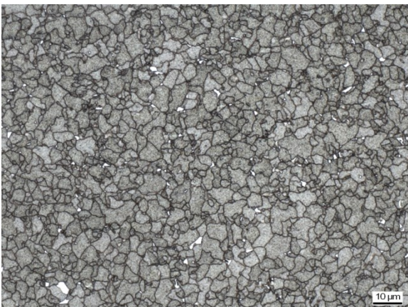
Abbildung C 113: WEZ Simulation (S 700MC, Blechdicke 10 mm), T_{\max}(1)=953,6^{\circ}\text{C} , t_{8/5}(1)=23,7\text{ s} , T_{\max}(2)=942,6^{\circ}\text{C} , t_{8/5}(2)=22,4\text{ s}
