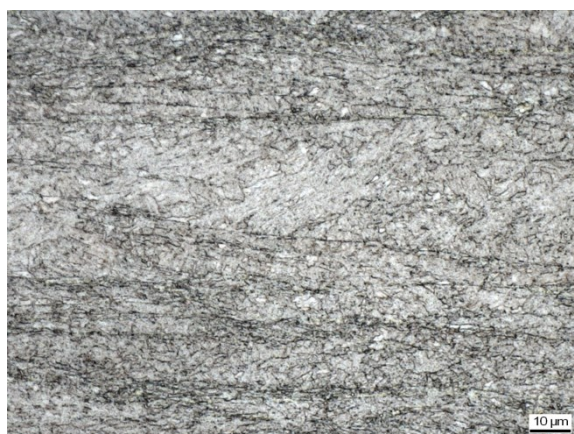
Abbildung C 108: WEZ Simulation (S 700MC, Blechdicke 10 mm), T_{\max}(1) = 728,7^{\circ}\text{C} , t_{8/5}(1) = 5,0 s, T_{\max}(2) = 734,6^{\circ}\text{C} , t_{8/5}(2) = 5,0 s
