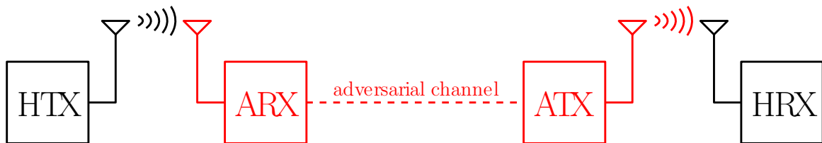
Figure 2.6.: Structure of the relay imposed by the attacker
