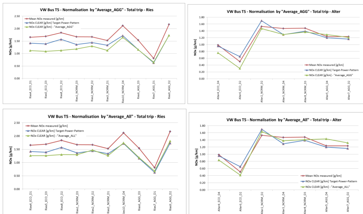
Figure 5-5: Normalisation results for NO x for VW Bus T5 (red: measured trip emissions, blue: weighted NO x with the “Standard CLEAR method”, green: weighted NO x by the “Extended CLEAR method”)
