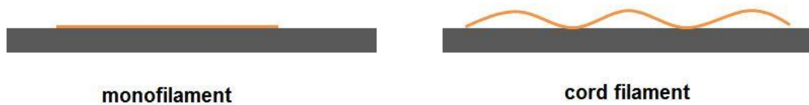
Figure 43: comparison of the sample contacting of monofilaments and cord filaments in SEM
