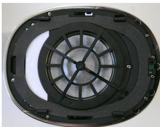
Figure 4.6: Headphones with microphone embedded in a rigid plastic hemisphere pointing away from the loudspeaker.
