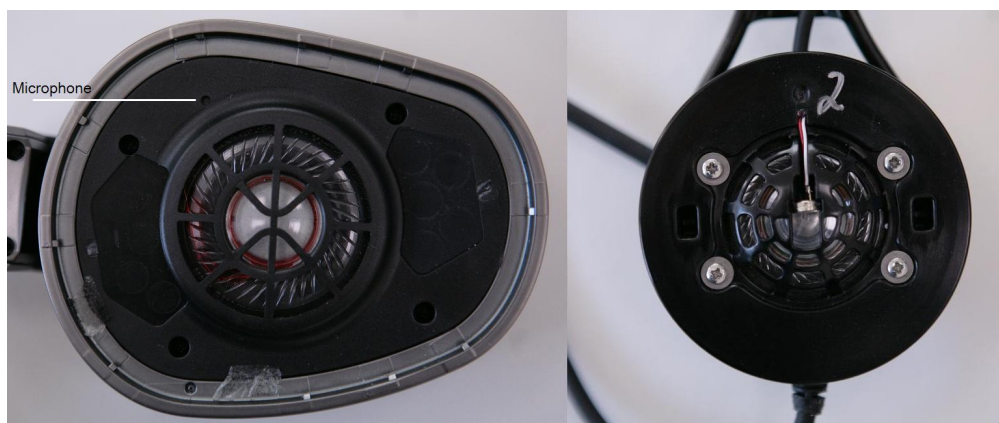
Figure 4.7: Headphones with different microphone positions. left: headphones with the microphone positioned next to the loudspeaker. right: aviation headset with the microphone positioned in a rigid hemisphere in a 90° angle to the loudspeaker.
