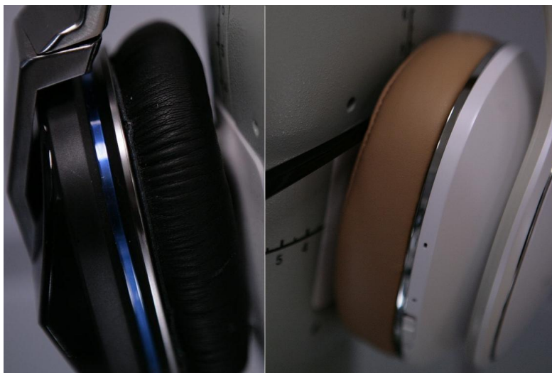
Figure 4.8: Misplacement of the headphones on a dummy head. Leakage can occur if the fit is not like intended. Glasses can also introduce leakage and lead to unfavorable reflections at the temples of the glasses [GMK05].
