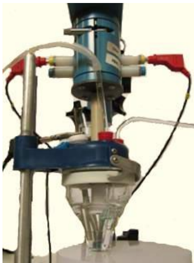
Figure 21: 3-electrode set-up for ex-situ electrochemical studies of the Pt-Co/C catalysts.
