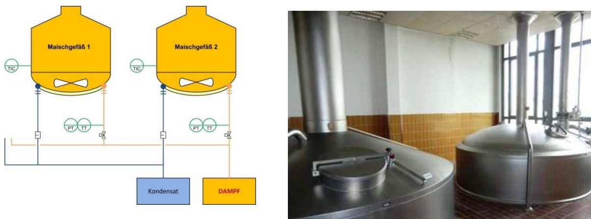
Figure 4-17: Mash tuns (schematic figure and real plant) supplied by steam (source: AEE INTEC)
