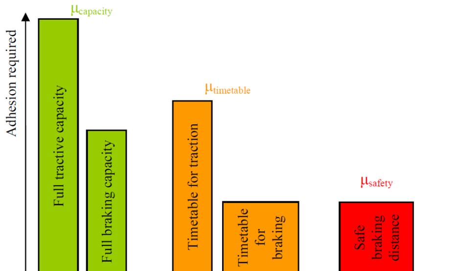
Figure 2.5: Common adhesion requirements in railway transportation<sup>9</sup>
