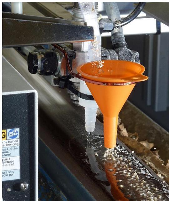
Figure 5.3: Conditioning with lubricant and sand without wheel load<sup>43</sup>
