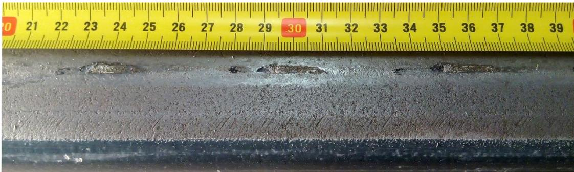
Figure 5.11: Strips on the rail caused by the stick-slip oscillation
