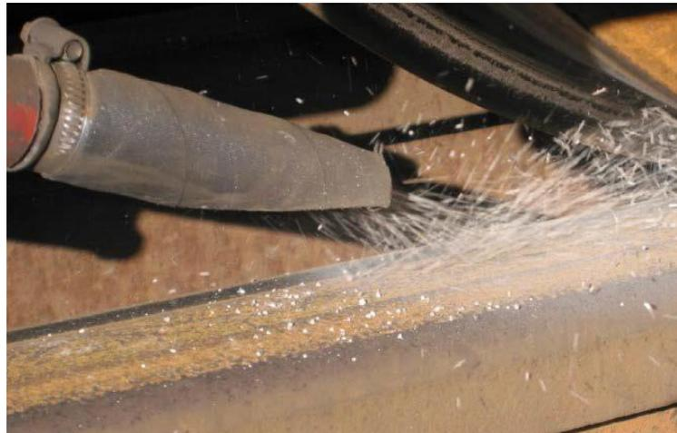
Figure 3.2: Sanding system in operation<sup>33</sup>
