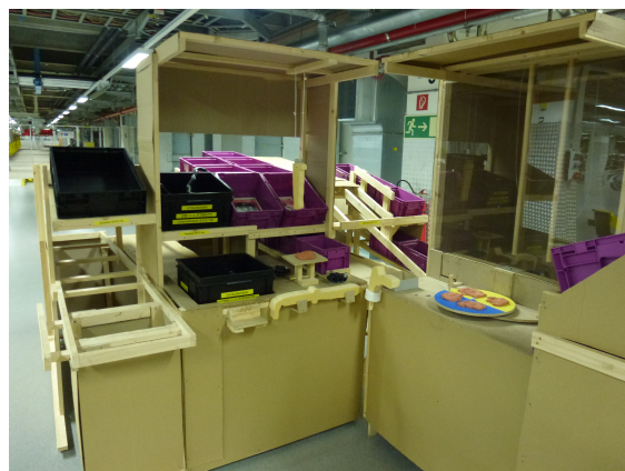
Figure 48.: Cardboard simulation at BMW Steyr
