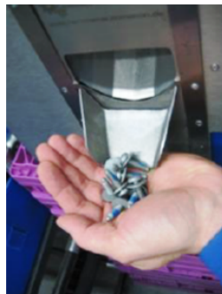
Figure 55.: Screw feeder with soap dispenser mechanism
