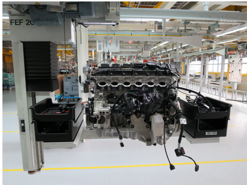
Figure 35.: Electric monorail system (EMS)
