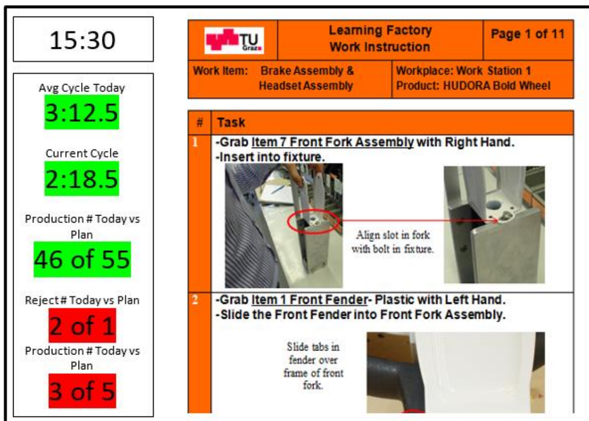
Figure 19: Display Screen at Work Station
