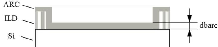
Figure 4.1: Parameter  $dbarc$  sets BARC thickness.
