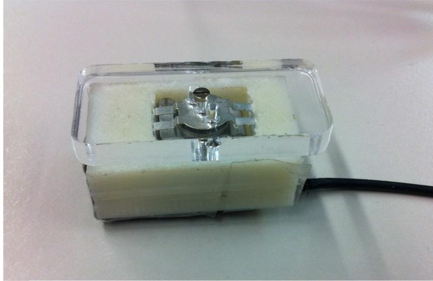
Figure A.4: Lateral view of the proposed EL device with electro-magnetic transducer (BHM BC2-E31) in the 3D printed housing with a mounted coupler disk on top.
