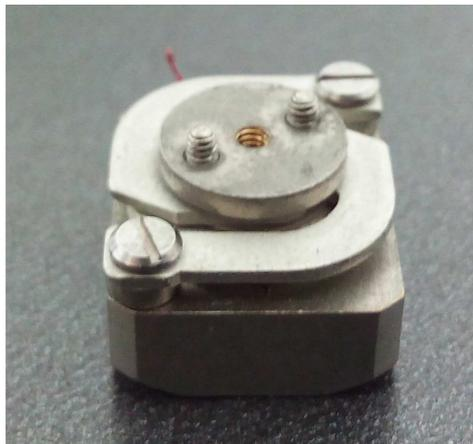
Figure A.1: Proposed electro-magnetic transducer (BHM BC2-E31).
