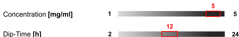
Figure 88 Optimized parameters for the acyl azide-PA adhesion system obtained via manual dip-coating.
