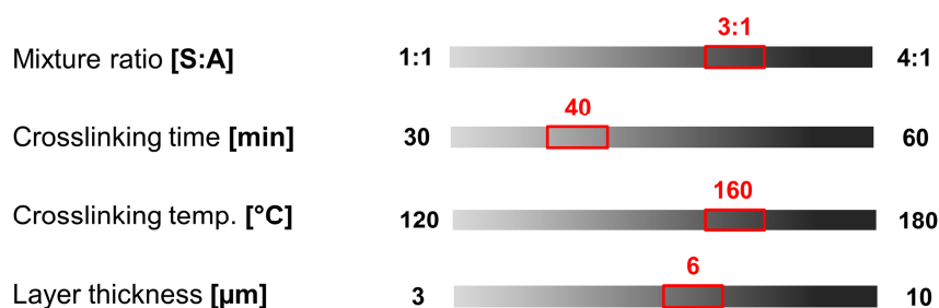
Figure 73 Optimized parameters for the adhesion system based on a mixture of polysulfide silanes (S 4 -Si) and aminosilanes (A) obtained via automated dip-coating.
