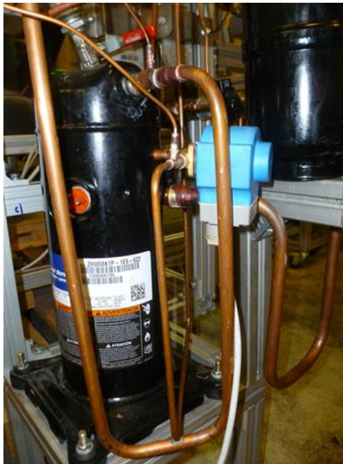
Figure 44: U-bend for preventing vibrations
