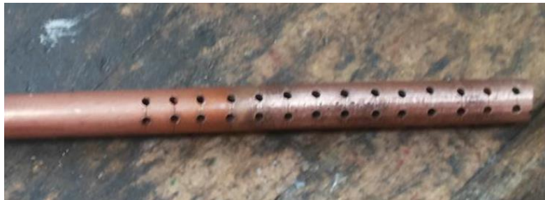
Figure 36: Distribution pipe of evaporator
