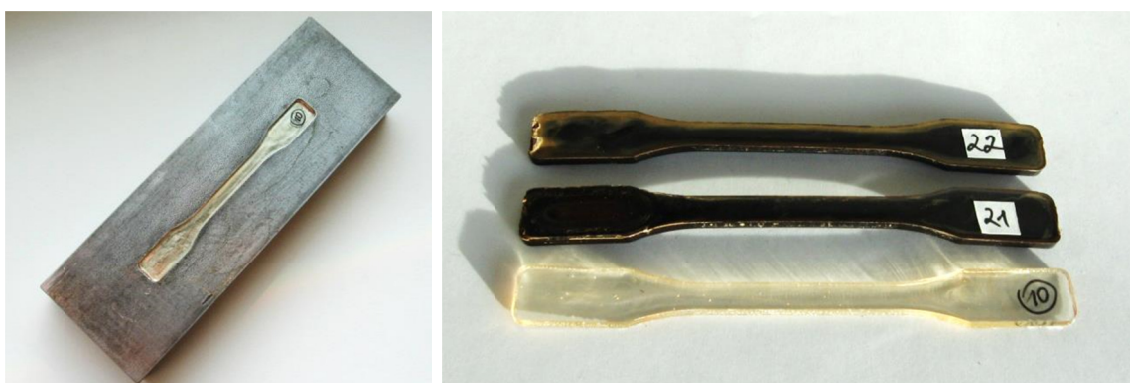
Figure 29. Steel mold for shouldered test bars (left) and prepared specimens (right), (neat DCPD (10), DCPD + 20 % wt NML (21) and DCPD + 30 % wt NML (22)).
