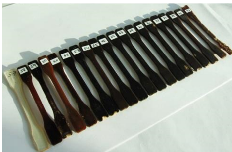
Figure 28. PDCPD shouldered test bars filled with insoluble lignin.
