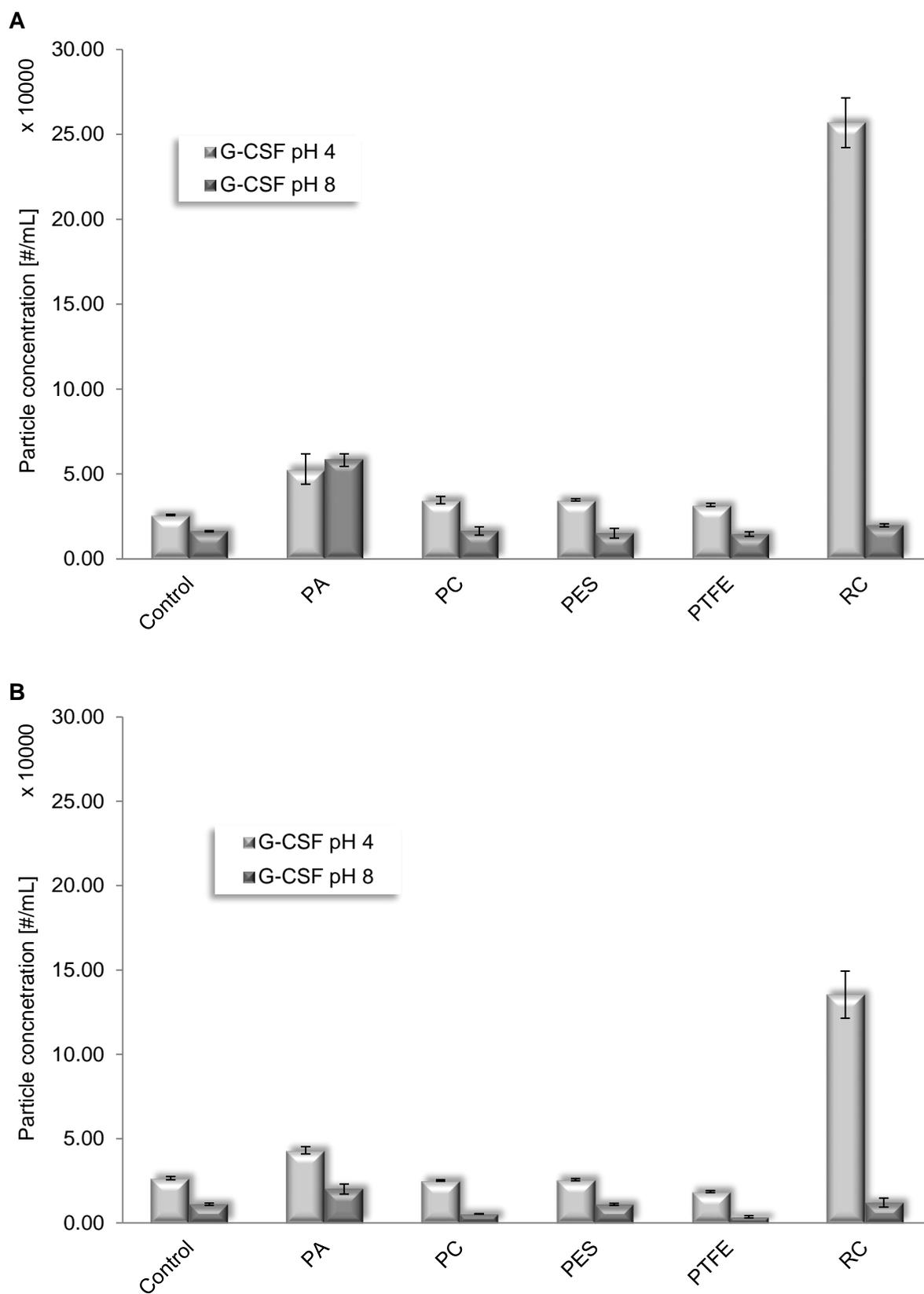
Figure 27: Results of MFI measurements from filter leachable stocks which were extracted at 30°C (A) and 50°C (B).
