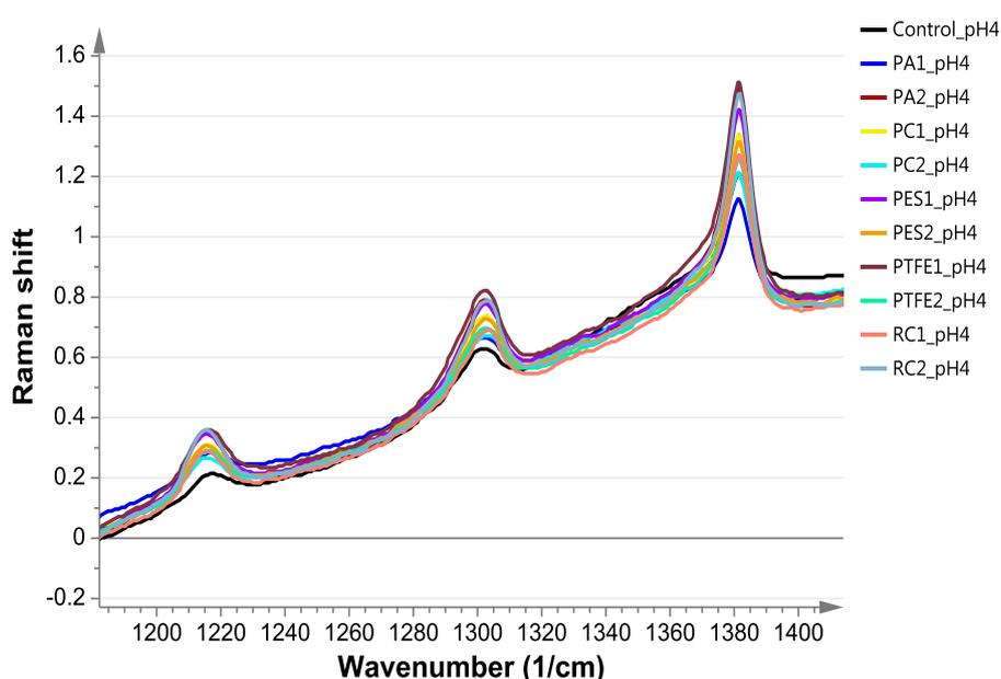
Figure 31: Results of the Raman spectroscopy analysis of G-CSF formulations spiked with pH 4 filter extracts extracted at 30°C.
