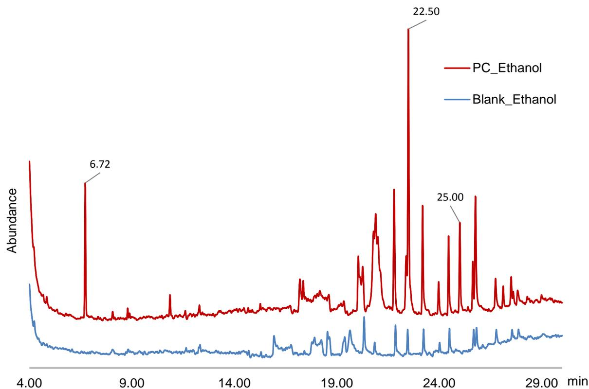
Figure 15: GC/MS total ion chromatogram of the polycarbonate-ethanol extract.
