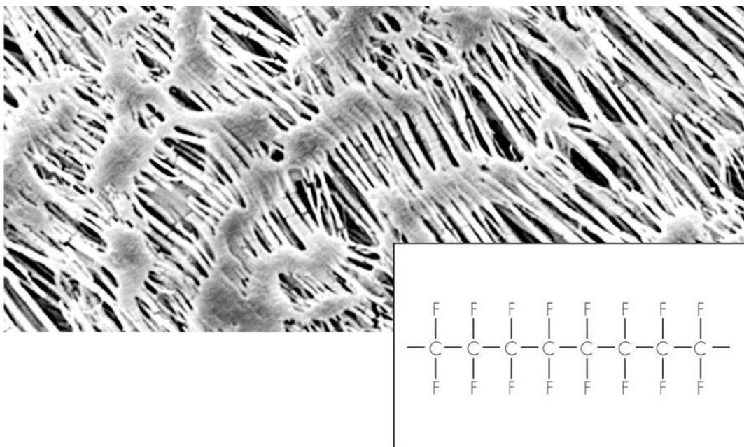
Figure 6: Microscopic image and structural formula of PTFE filter membranes [22].
