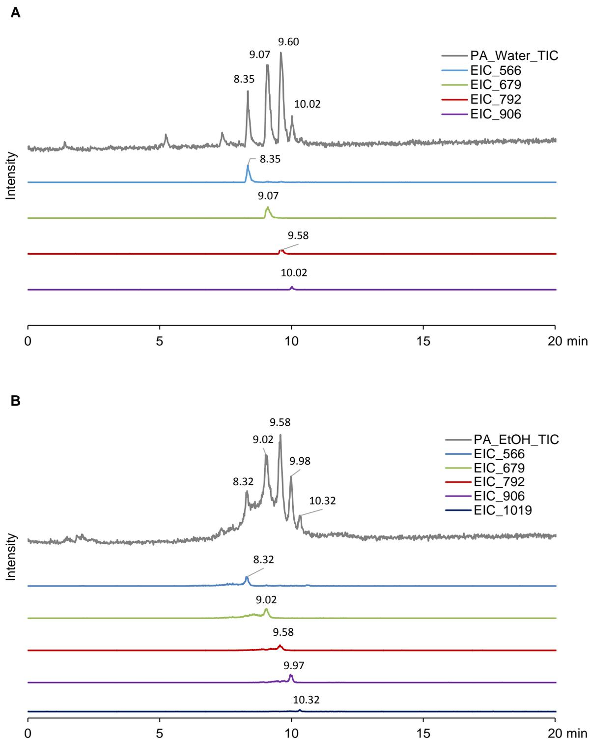
Figure 21: HPLC/MS chromatograms of the polyamide-water (A) and the polyamide-ethanol (B) extract. The upper chromatogram is the total ion current (TIC) chromatogram of the extract; the remaining chromatograms are extracted ion chromatograms at the indicated mass value.
