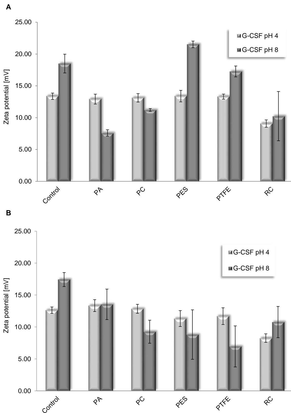
Figure 30: Results of zeta potential analysis from filter leachable stocks which were extracted at 30°C (A) and 50°C (B).
