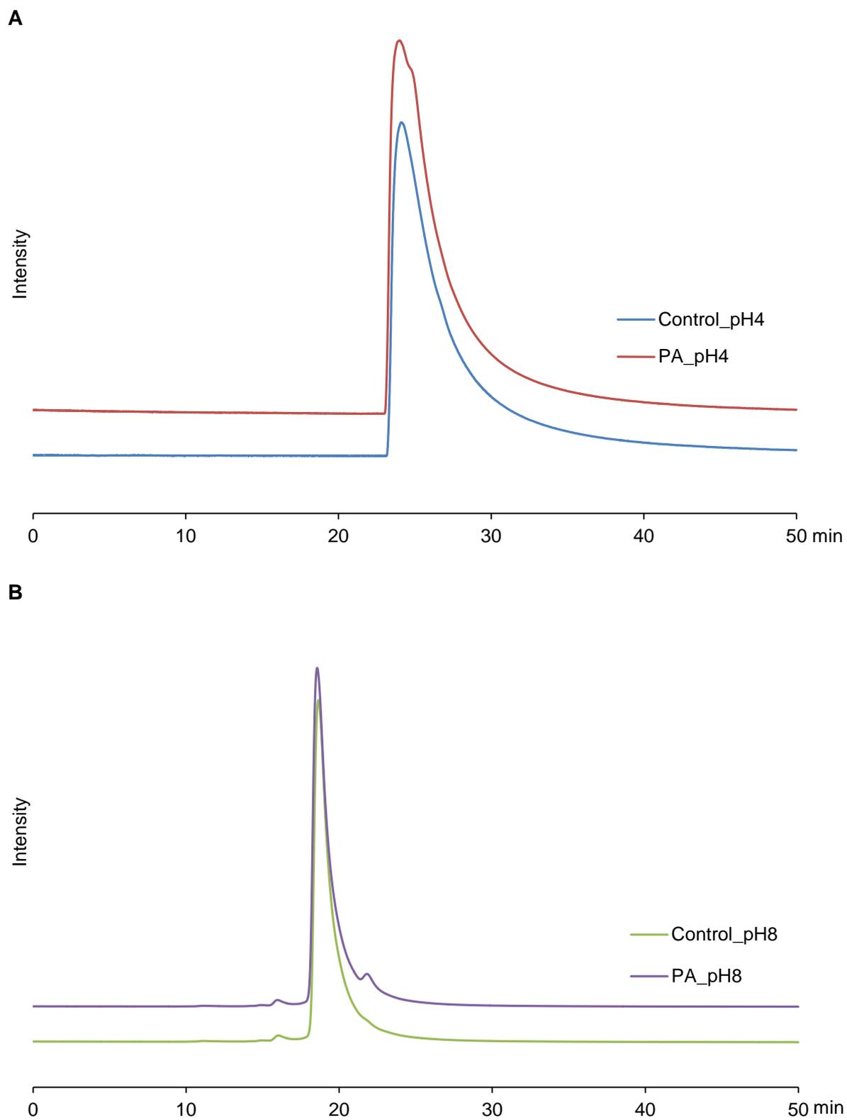
Figure 29: SEC chromatograms of the control and the polyamide samples at pH 4 (A) and pH 8 (B).
