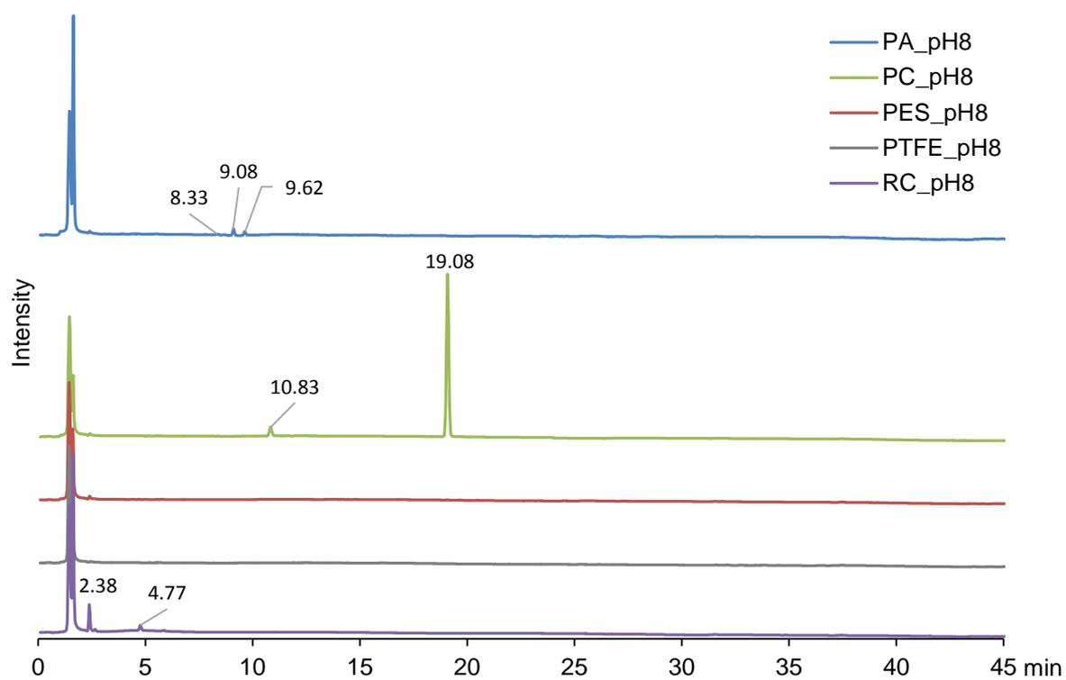
Figure 24: HPLC/UV chromatograms of the different filter extracts at pH 8 for the leachable study.
