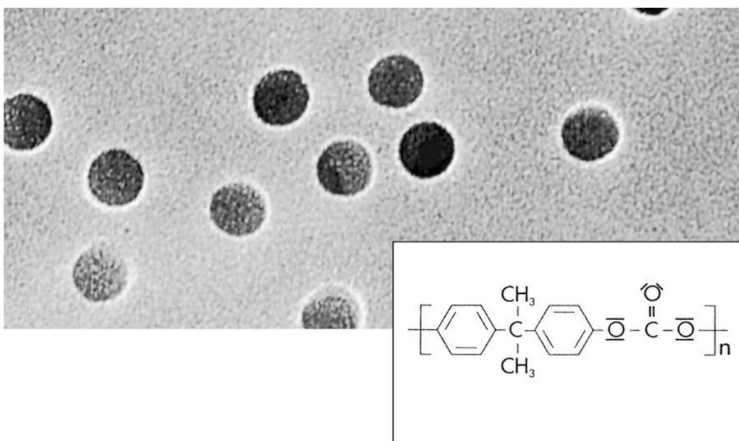
Figure 4: Microscopic image and structural formula of PC filter membranes [16].
