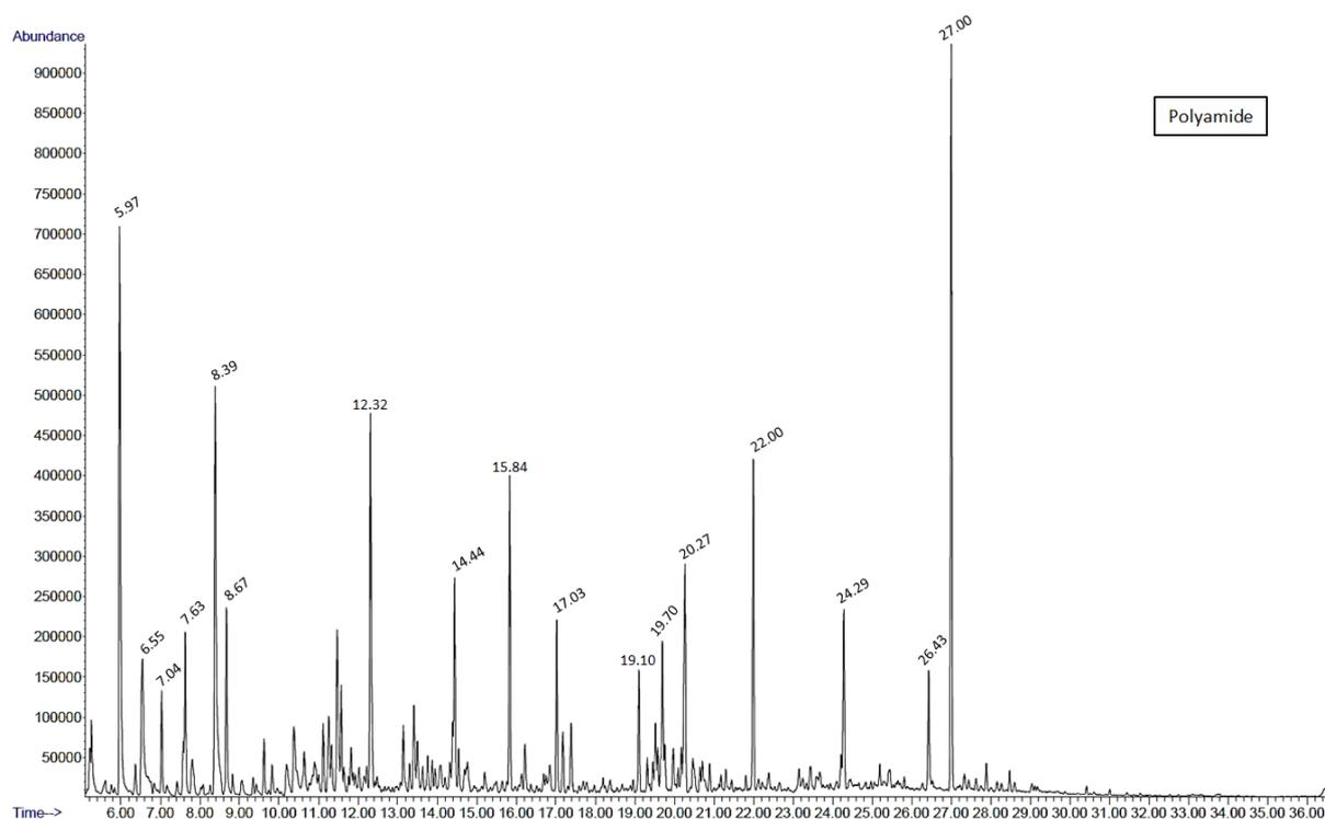
Figure 9: SPME-HS-GC/MS total ion chromatogram of polyamide filters.
