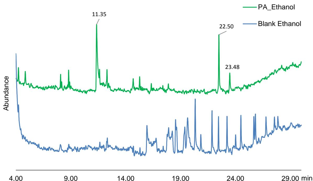
Figure 14: GC/MS total ion chromatogram of the polyamide-ethanol extract.
