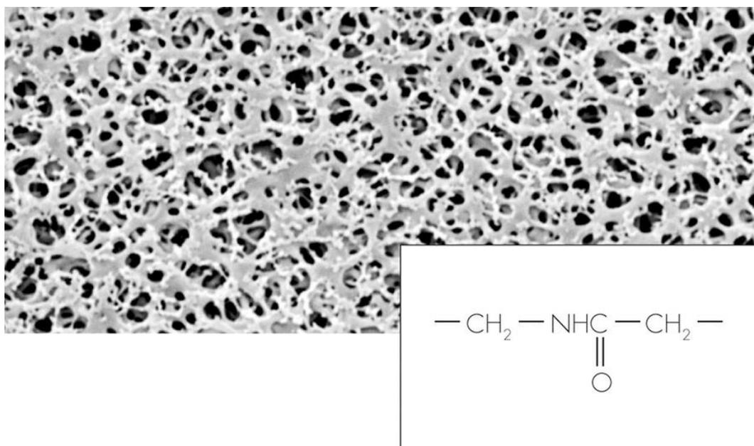
Figure 3: Microscopic image and structural formula of PA filter membranes [14].
