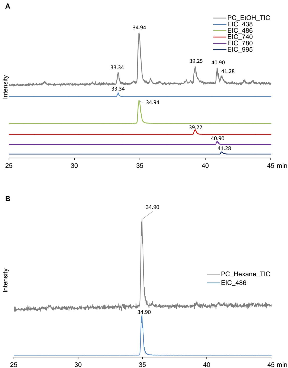
Figure 22: HPLC/MS chromatograms of the polycarbonate-ethanol (A) and the polycarbonate-hexane (B) extract. The upper chromatogram is the total ion current (TIC) chromatogram of the extract; the remaining chromatograms are extracted ion chromatograms at the indicated mass value
