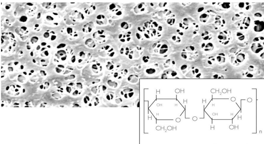
Figure 7: Microscopic image and structural formula of RC filter membranes [25].
