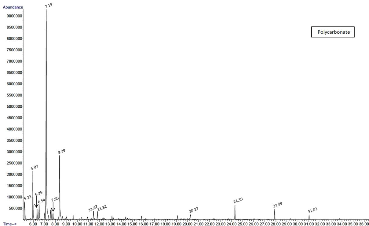
Figure 10: SPME-HS-GC/MS total ion chromatogram of polycarbonate filters.
