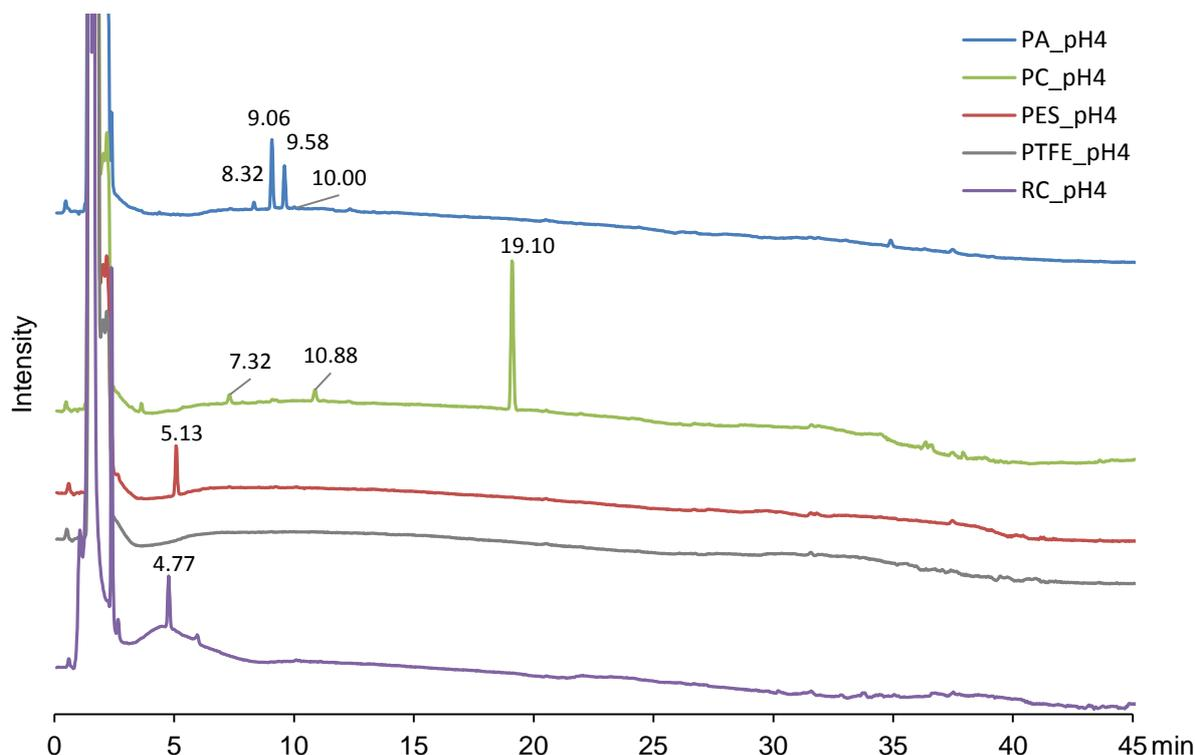
Figure 23: HPLC/UV chromatograms of the different filter extracts at pH 4 for the leachable study.
