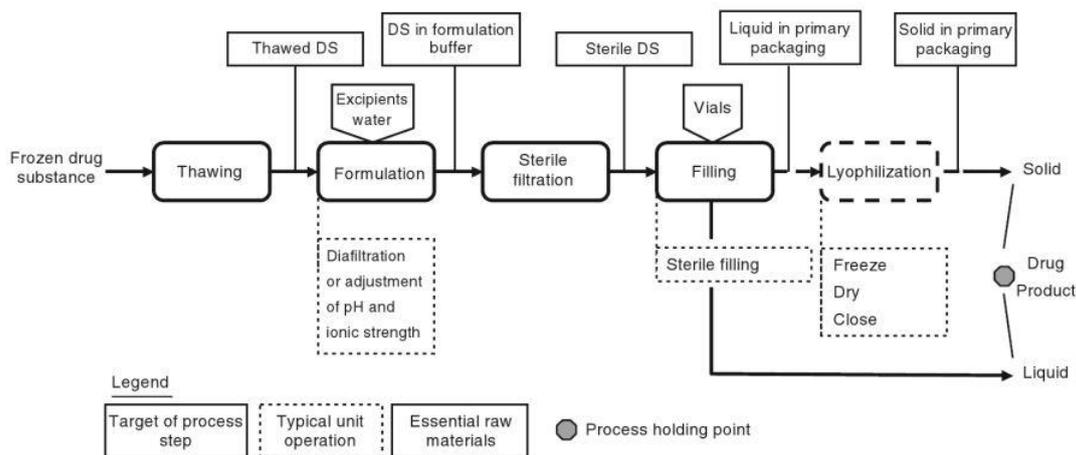
Figure 1: Schematic of formulation and filling of pharmaceutical proteins. DS = drug substance [2].
