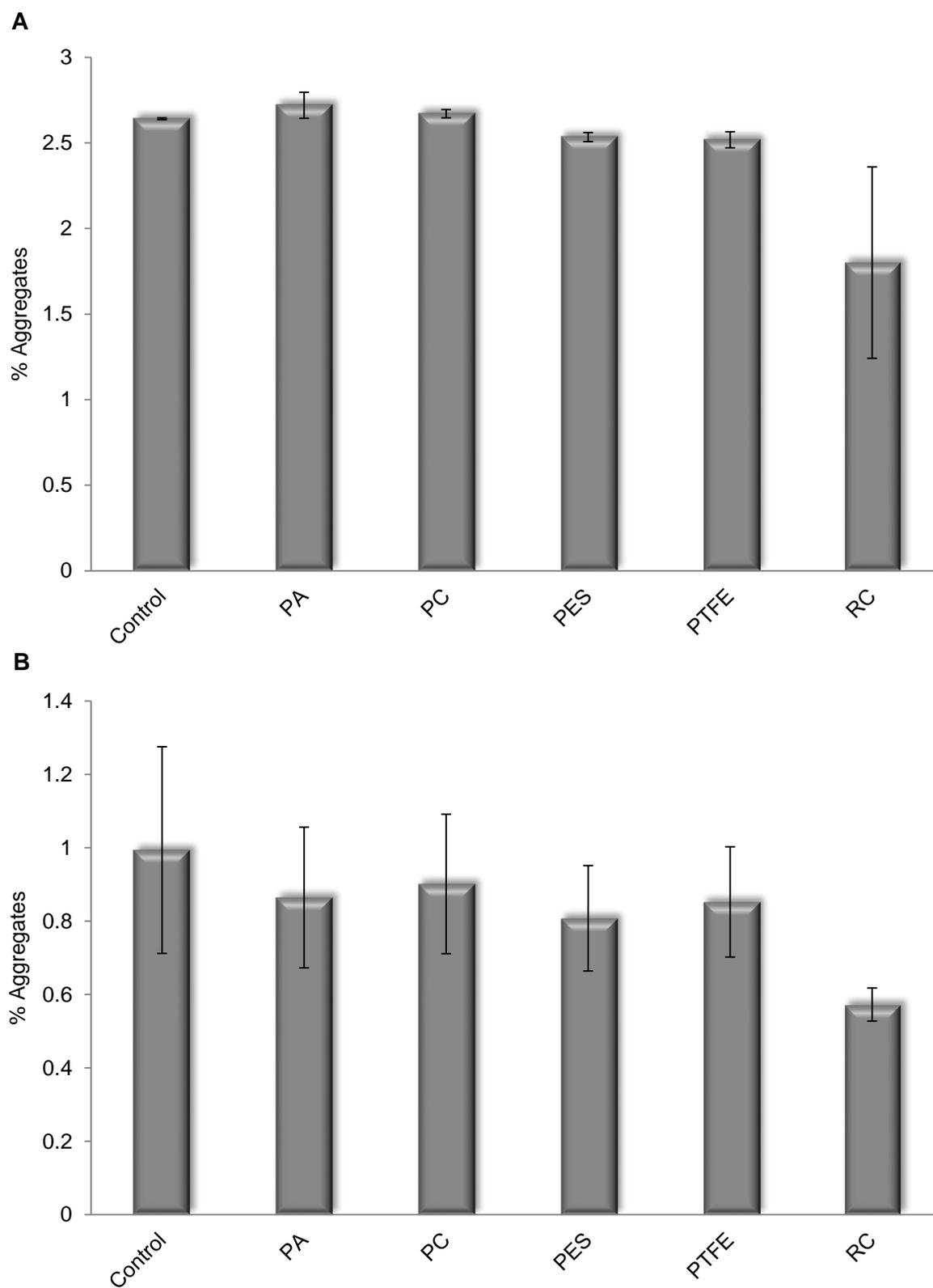
Figure 28: Aggregate levels in G-CSF formulations at pH 8 analyzed by SEC-HPLC after spiking with filter leachable stocks which were extracted at 30°C (A) and 50°C (B).
