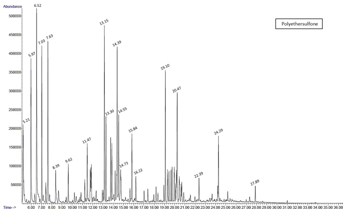
Figure 11: SPME-HS-GC/MS total ion chromatogram of polyethersulfone filters.
