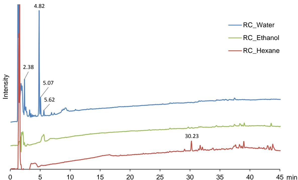
Figure 20: HPLC/UV chromatograms of the regenerated cellulose extracts from the CES.
