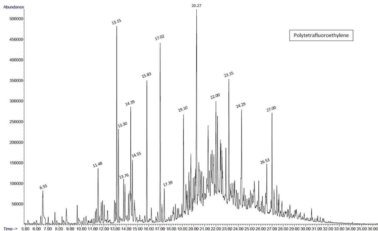
Figure 12: SPME-HS-GC/MS total ion chromatogram of polytetrafluoroethylene filters.
