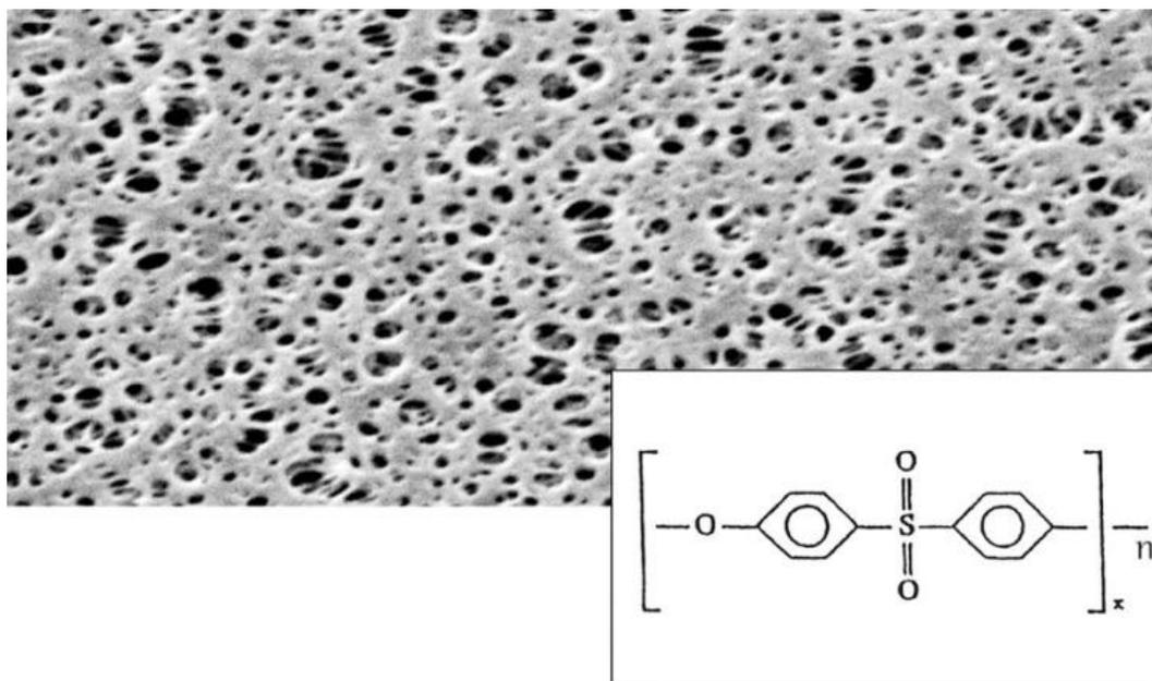
Figure 5: Microscopic image and structural formula of PES filter membranes [19].
