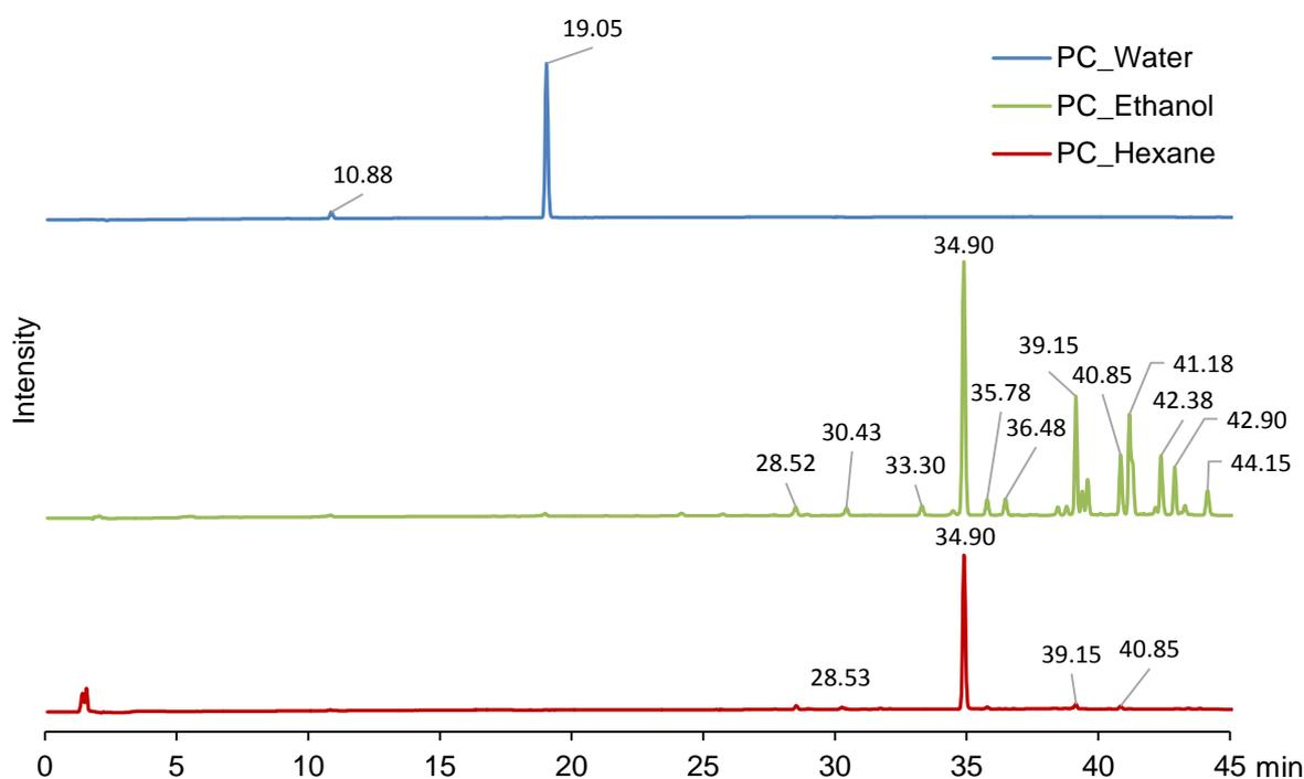
Figure 17: HPLC/UV chromatograms of the polycarbonate extracts from the controlled extraction study.
