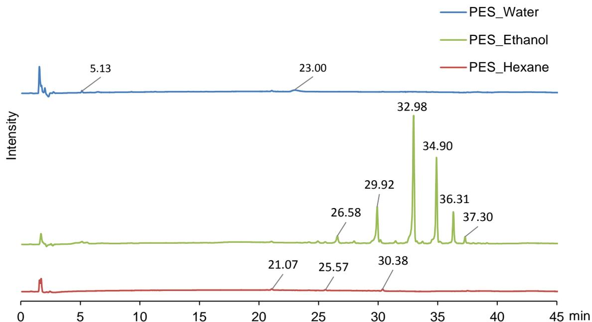
Figure 18: HPLC/UV chromatograms of the polyethersulfone extracts from the CES.
