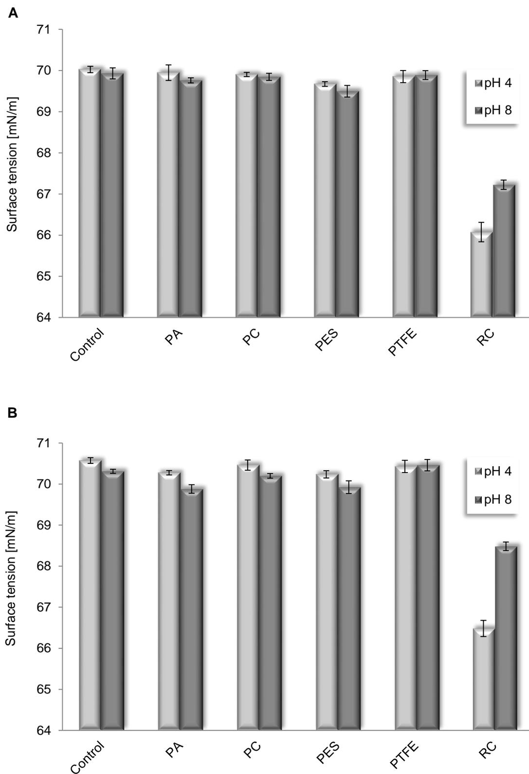
Figure 26: Results of surface tension measurements from filter leachable stocks which were extracted at 30°C (A) and 50°C (B).
