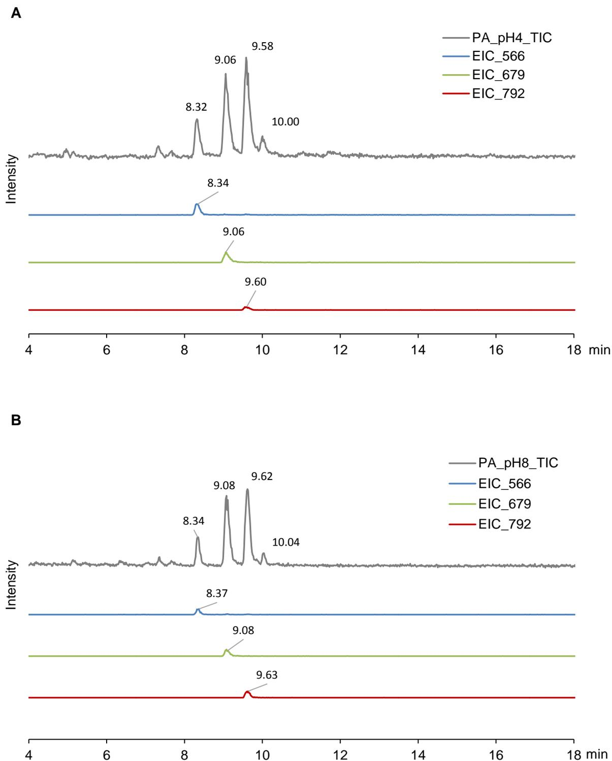
Figure 25: HPLC/MS chromatograms of the polyamide-CP-buffer pH 4 (A) and the polyamide-CP-buffer pH 8 extract. The upper chromatogram is the total ion current (TIC) chromatogram of the extract; the remaining chromatograms are extracted ion chromatograms at the indicated mass value.
