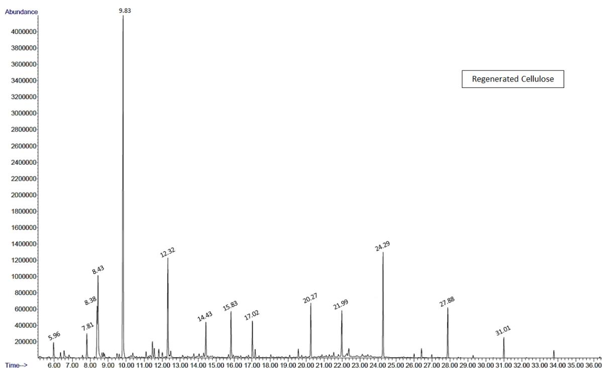
Figure 13: SPME-HS-GC/MS total ion chromatogram of regenerated cellulose filters.
