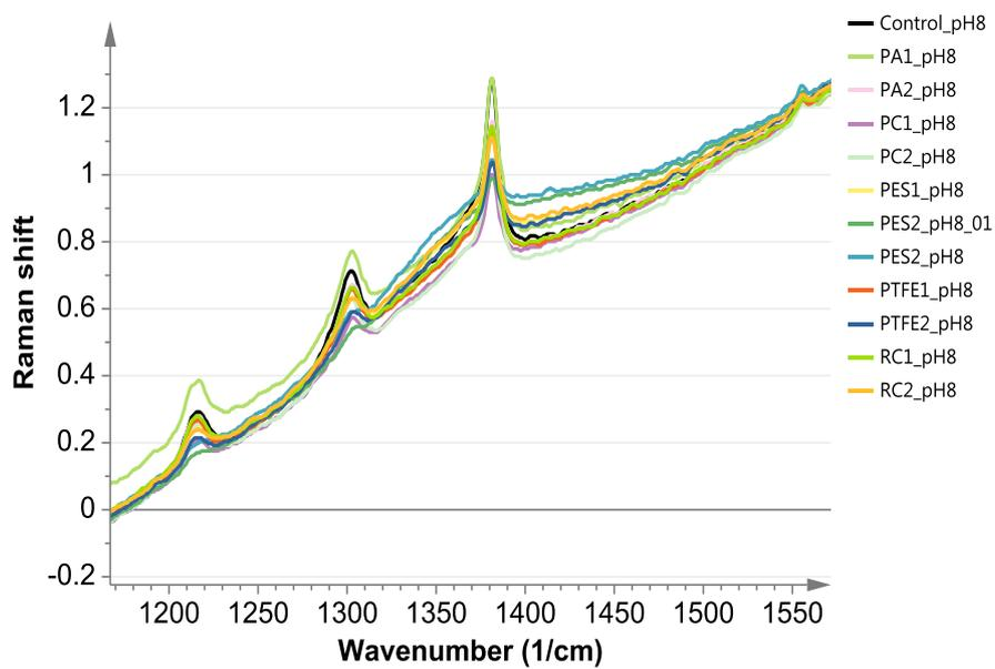
Figure 32: Results of the Raman spectroscopy analysis of G-CSF formulations spiked with pH 8 filter extracts extracted at 30°C.
