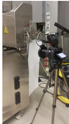
Figure 17: Set-up for optical RTD measurements
