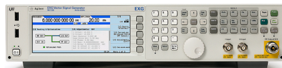
Figure 5.18: EXG N5172B Front Panel [36]
