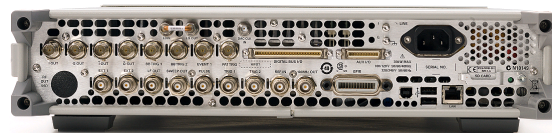
Figure 5.19: EXG N5172B Back Panel [36]
