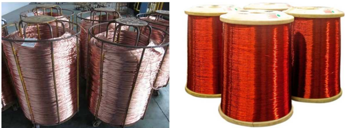
Figure 1: Raw wire and enameled copper wire (source MAG)
