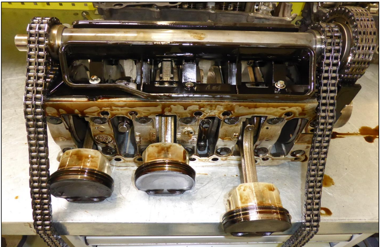
Fig. 26: Crank train with intermediate shaft at Porsche 986
