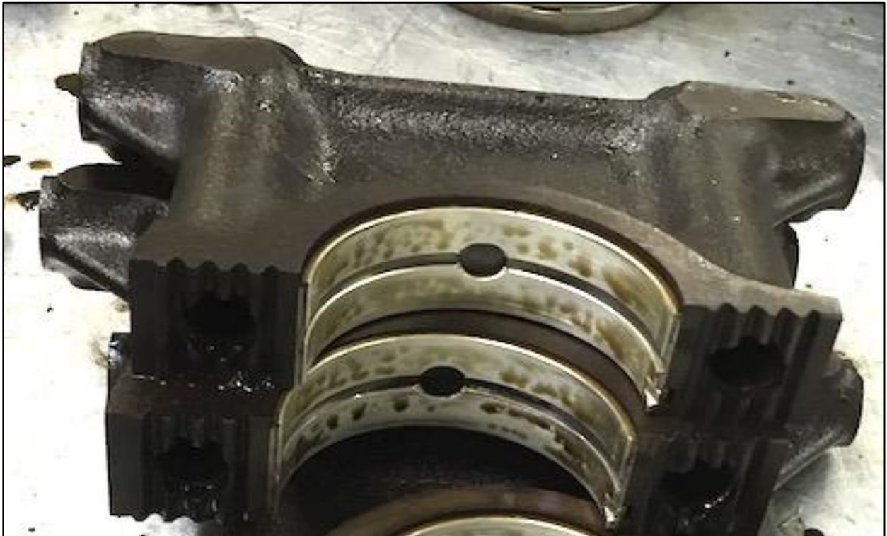
Fig. 21: Bearing bridges at Alfa Romeo 33
