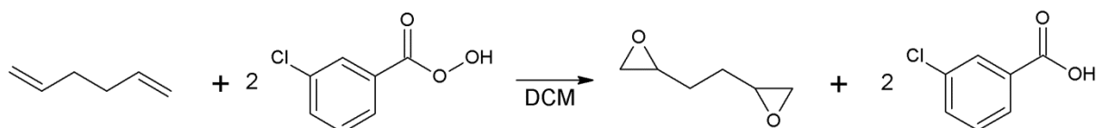
Scheme 24: Reaction scheme for epoxidation of 9c with m CPBA.
