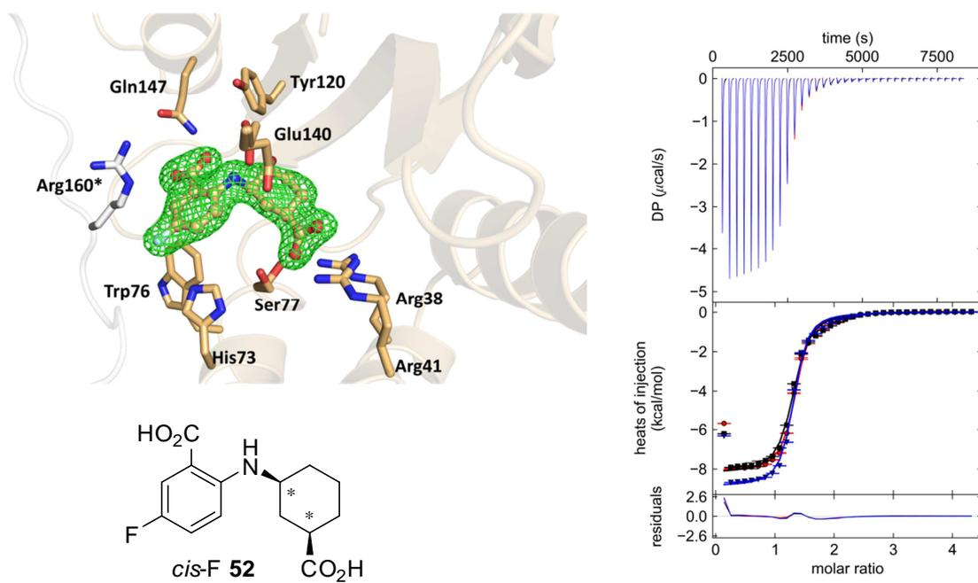
Figure 140: Crystal structure of *cis*-F-Phenazistatin **52** and its ITC curve.
