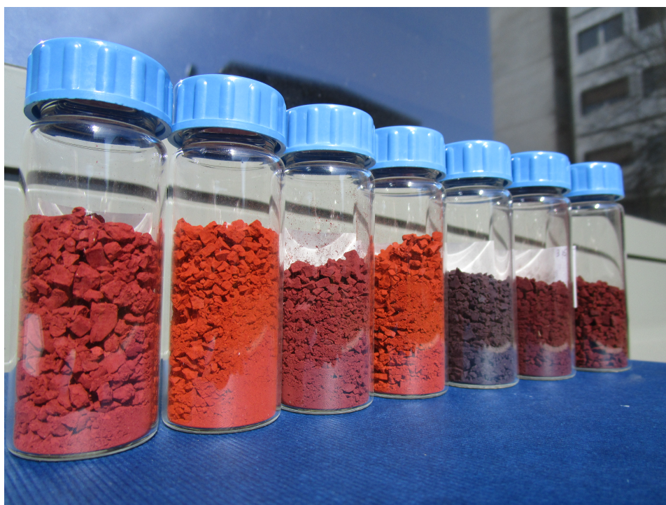
Figure 4.22: Oxygen Carriers synthesised with Pre. From left to right: Fe-Ce, Fe-Al-Ce, Fe-Zr, Fe-Al-Zr, Fe-Cu, Fe-Al-Cu (16 h), Fe-Al-Cu (3 h)
