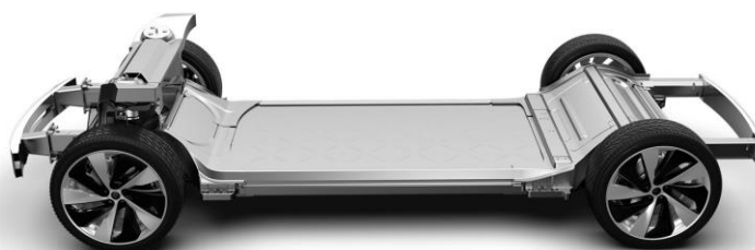
Figure 38 Variable Platform Architecture used for all vehicles (Faraday Future Inc., 2016d)
