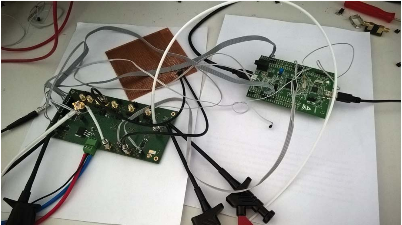
Figure 5.10. Picture of the time interleaved measurement setup, with channel 4 under test, with the micro controller-board all connections respectively.
