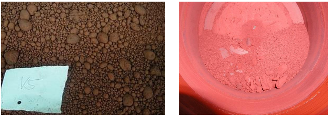
Figure 25: Left: the particle size distribution of the sample V5 induced by the binder Optapix PAF 2. Right: reactor vessel with a solid dense layer at the wall and bottom.
