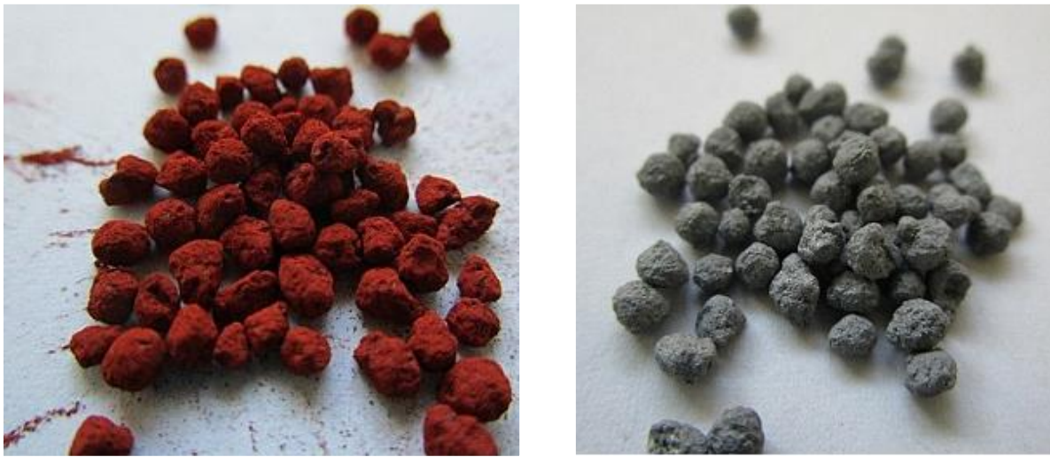
Figure 26: Sample V7 with a composition of 90 wt% \text{Fe}_2\text{O}_3 and 10 wt% \text{Al}_2\text{O}_3 with a diameter of 1 – 2 mm. Fresh sample (left) and after cyclic experiments (right).
