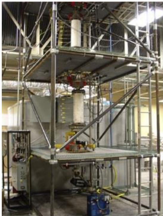
Figure 17: Left: photo of the 25 kW th sub-pilot SCL unit at The Ohio State University. 112 £ Right: schematic representation of the two-compartment fluidized-bed reactor proposed by Rydén et al.. 135 ££
