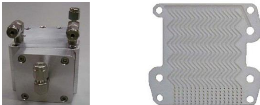
Figure 18: Left: the CLSR micro-reactor proposed by Moghtaderi. Right: a single reactor plate with the zigzag shaped pattern, which are used in the CLSR micro-reactor. 146 £££
