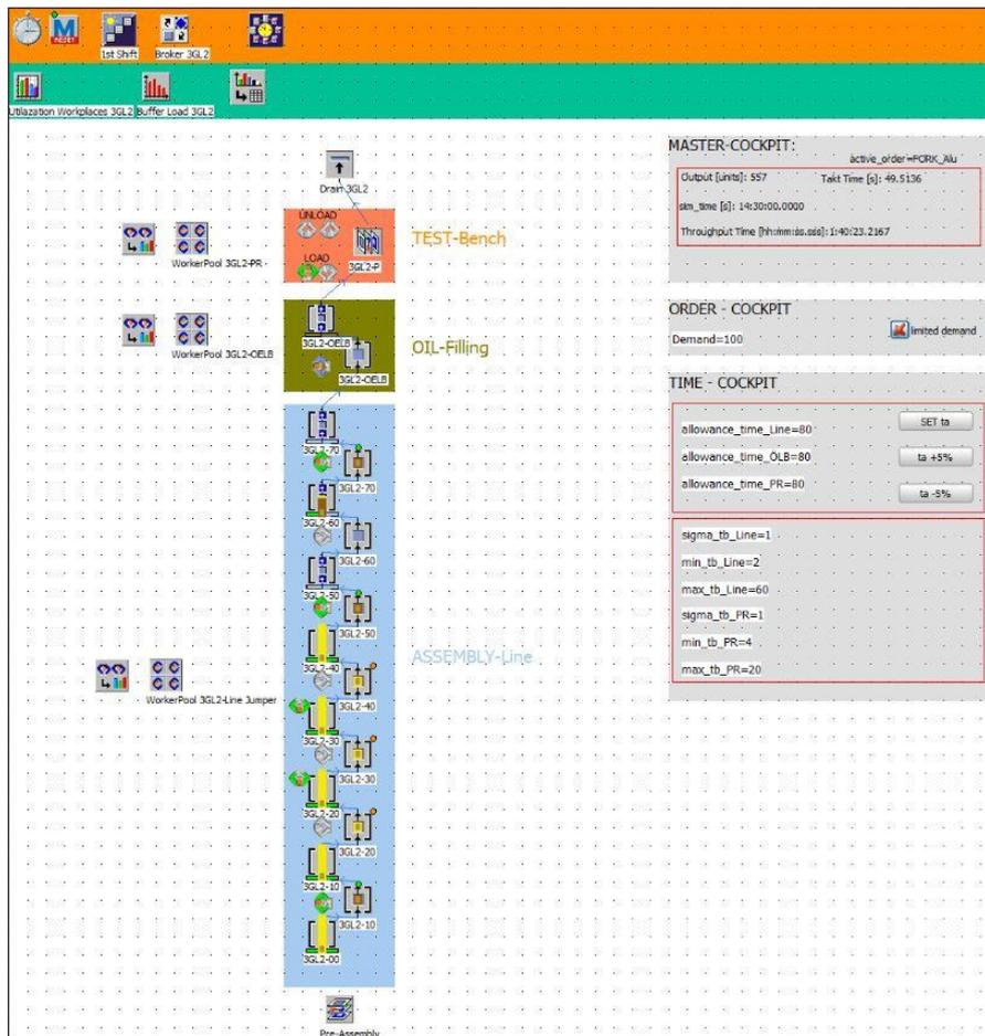
Figure 3.32: Screenshot of the simulation model of the current production system
