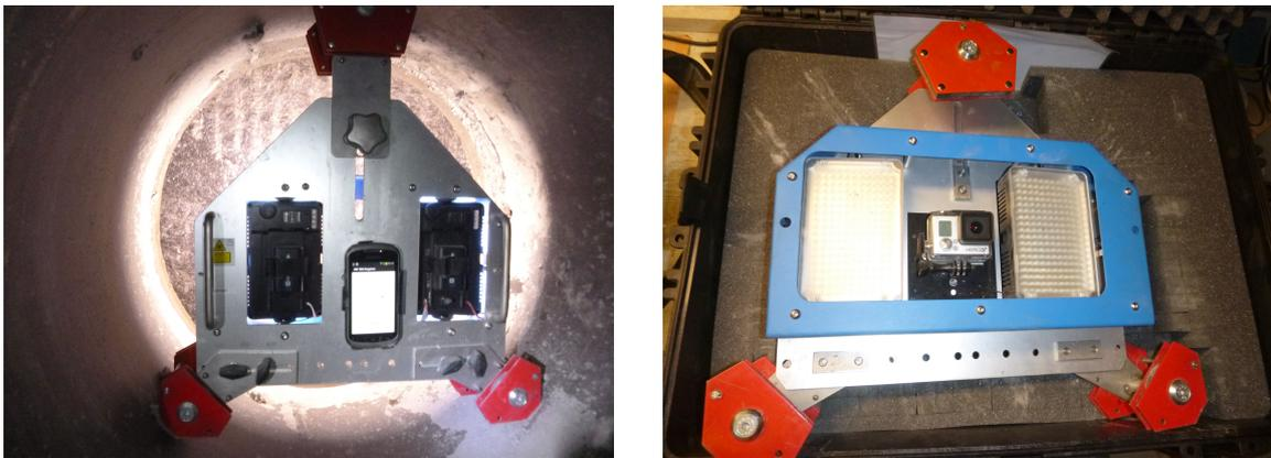
Figure 2.1: Imaging unit with smartphone, outdoor camera, LED lamps and laser pointers
