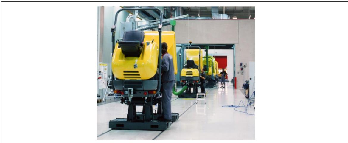
Figure A - 2 : Dumper assembly line at Wacker Neuson Linz GmbH, source: Wacker Neuson (2016)., modified
