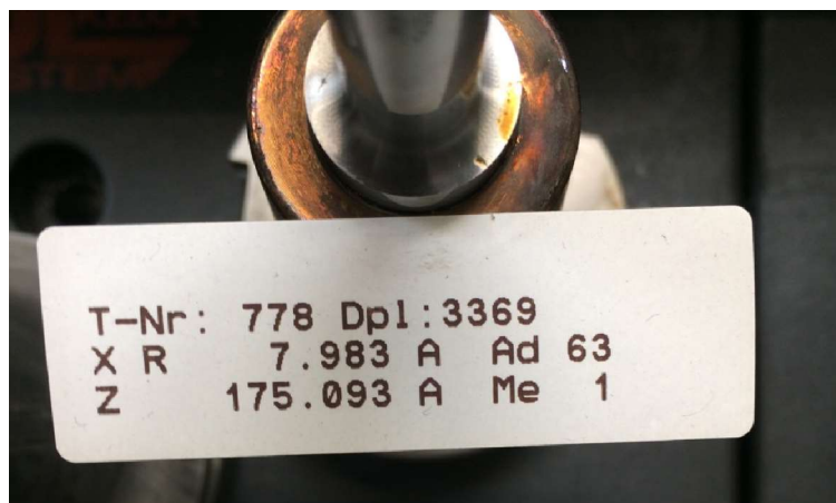
Figure 36: Geometry correction printed on a sticker, source: BRP-Rotax (2016) internal source
