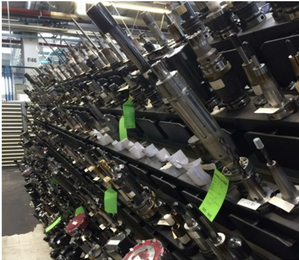
Figure 34: Interim tool storage at the pre-setting area, source: BRP-Rotax (2016), internal source
