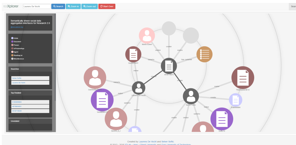
Figure 5.23: Situation when Selver Softic and Laurens de Vocht have been searched by keywords. The found connection is the common paper. The connection is populated when the paper is clicked.
