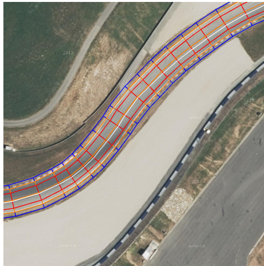
Figure 3.5: Road graph refinement. OSM data is shown as white polyline, the optimized road surface area is enclosed by smoothly connected orange quads.
