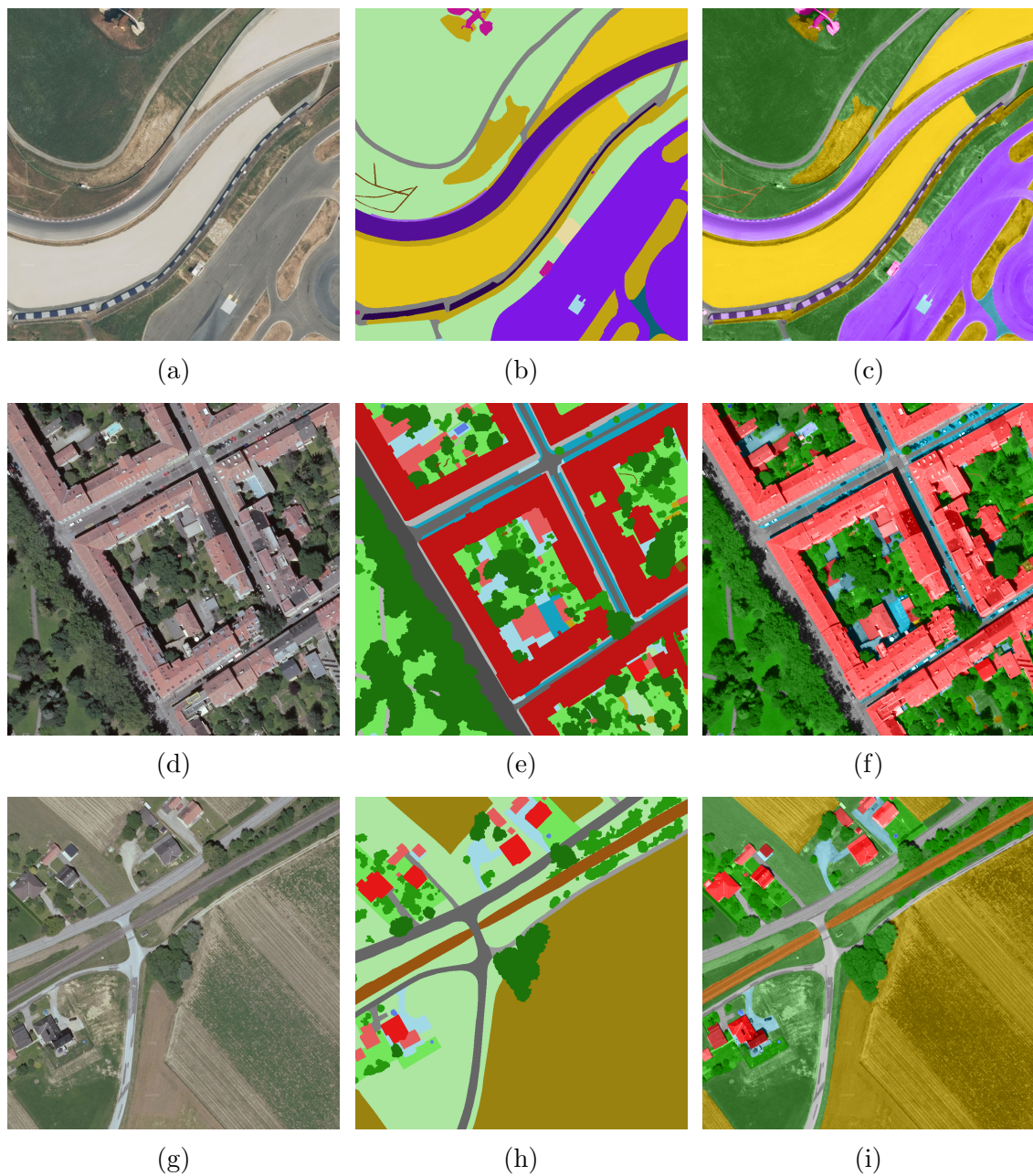
Figure A.1: Examples of labeled ground truth data (II). The first column contains the original aerial images a , the second column the manually created segmentation. An overlay of both images is shown in the third column. Top row (a-c): Section of the Red Bull Ring race track. Middle row (d-f): City center of Graz, Austria. Bottom row (g-i): Rural area, Styria, Austria.
