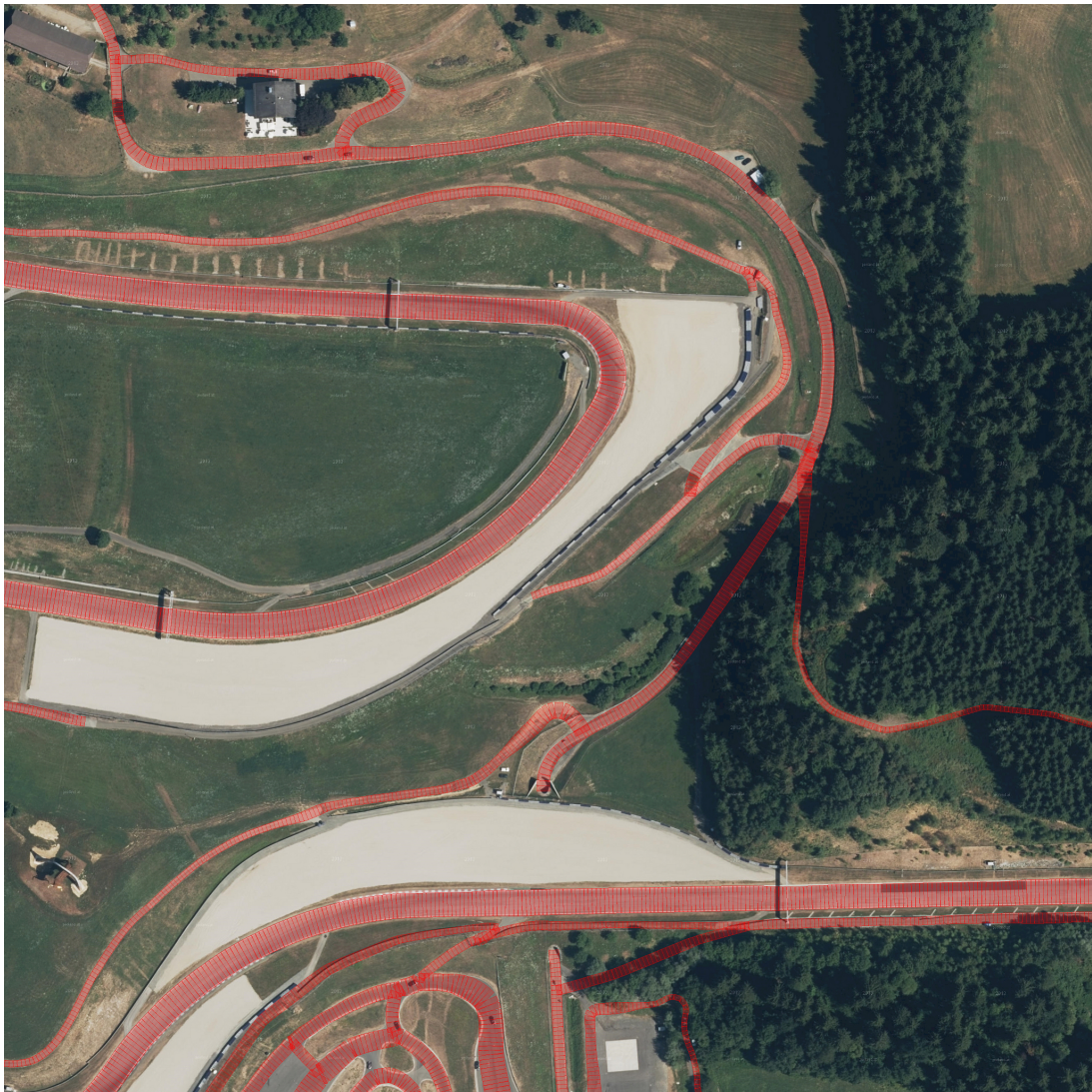
Figure 3.8: Example output of our algorithm: A road graph for a region of 0.26 \text{ km}^2 after the NLO-based refinement. All connections between road segments are preserved.
