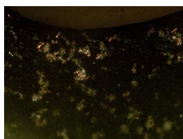
Figure 4-28 PLM after 20' dissolution testing
