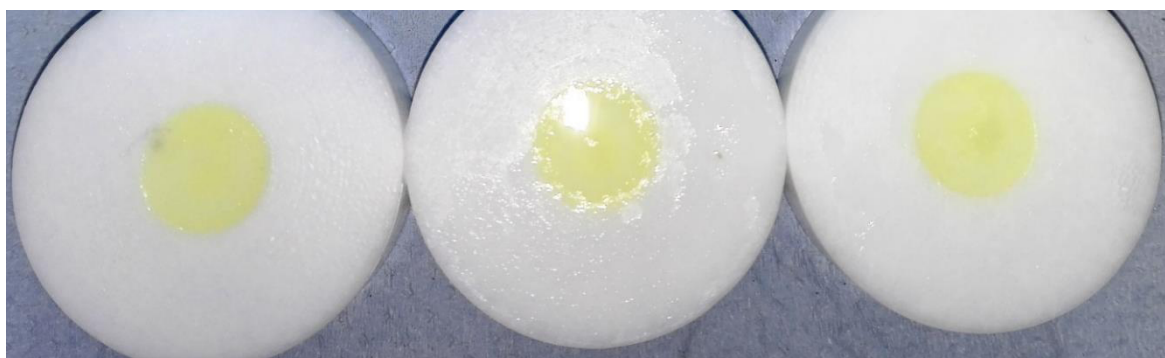
Figure 6-33 10% API with 2:3 EE:HPMC; picture taken after dissolution testing (70')
