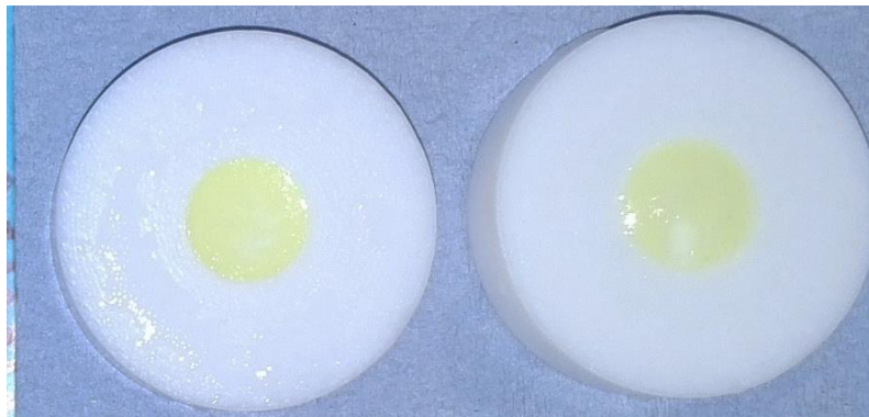
Figure 6-28 10% API with 2:1 EE:HPMC; picture taken after dissolution testing (70')
