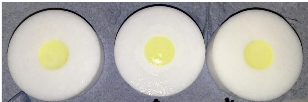
Figure 6-29 10% API with 3:2 EE:HPMC; picture taken after dissolution testing (70')
