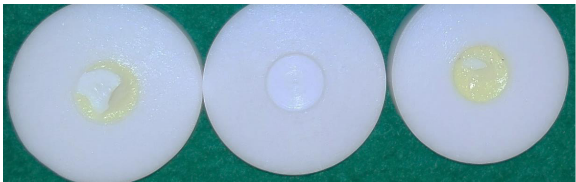
Figure 6-27 10% API with 4:1 EE:HPMC; picture taken after dissolution testing (70')
