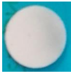
Figure 4-25 VCM prepared sample of HPMC (pure polymer)
