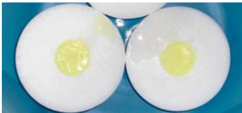
Figure 6-34 10% API 1:1 EE:HPMC; picture taken after dissolution testing (70')
