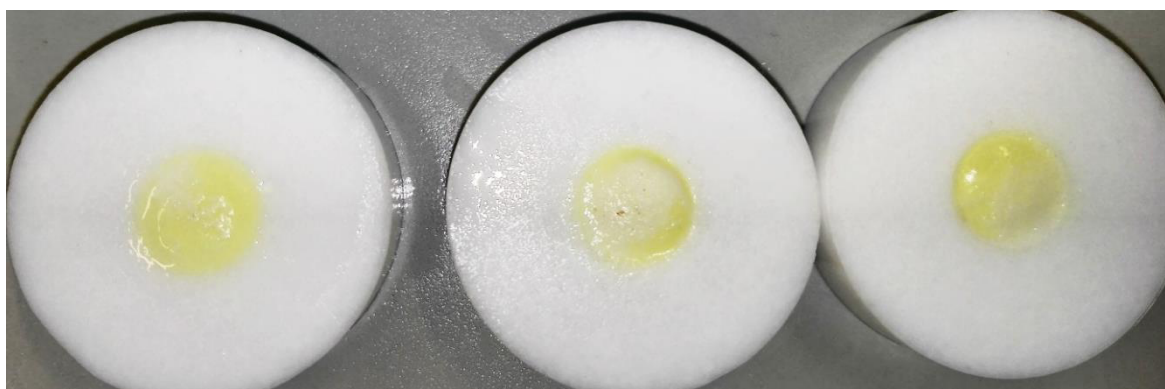
Figure 6-30 10% API with HPMC; picture taken after dissolution testing (70')
