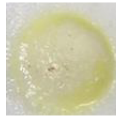
Figure 4-26 VCM prepared sample of NMD (10 %) and HPMC (90 %) after dissolution testing
