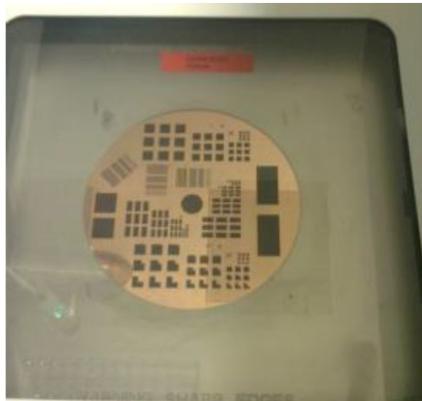
FIGURE 1.12: Wafer with test structures on the printer pallet, surrounded by the shim.
