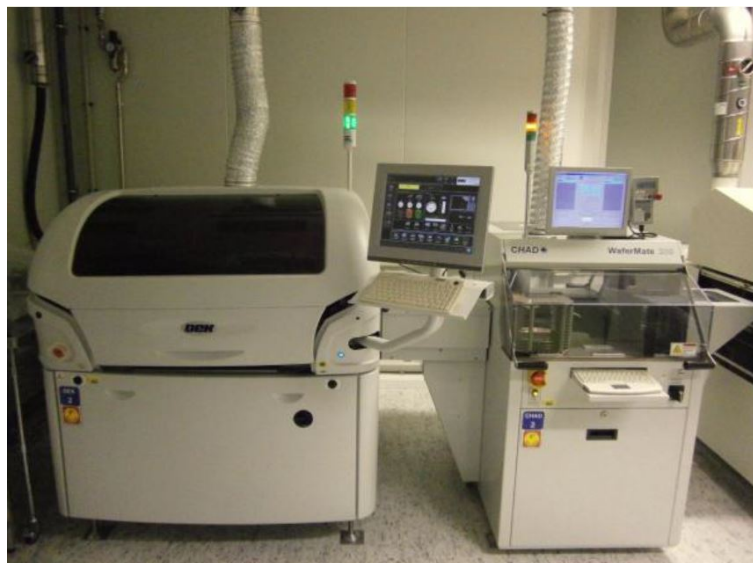
FIGURE 1.11: Used printing equipment DEK Horizon i02 with WaferMate 200 wafer handler from CHAD Industries.
