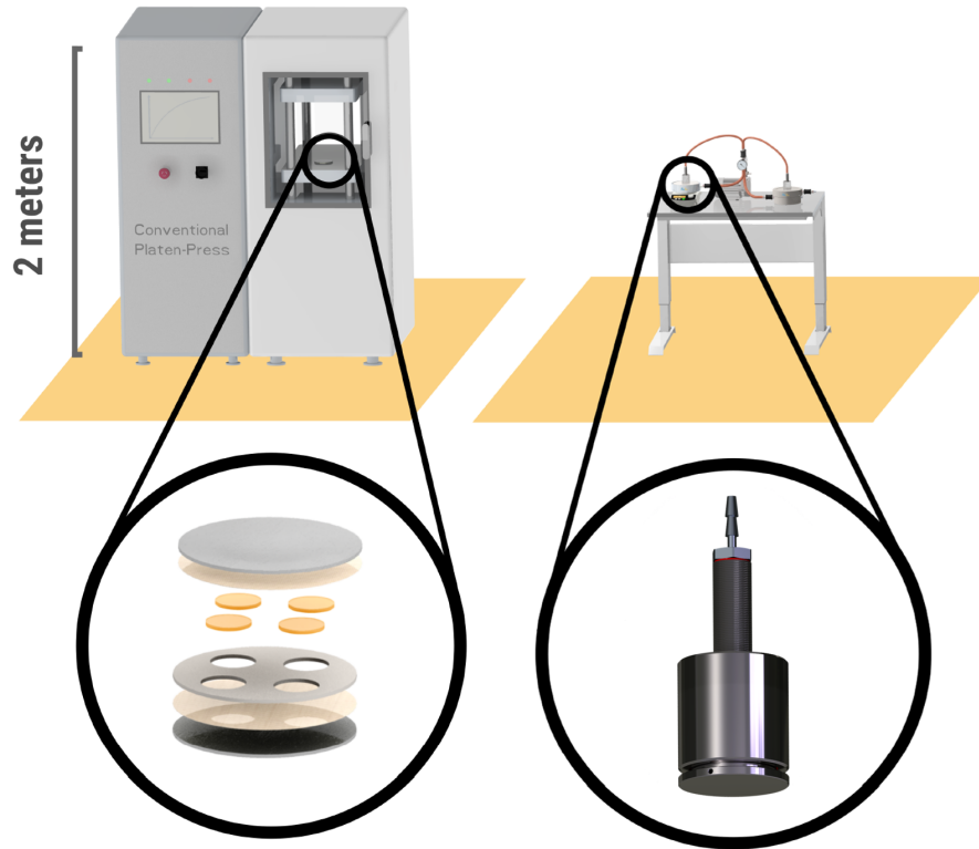
Figure 30 : Size comparison between the VCM setup and a conventional platen press(MeltPrep GmbH)
