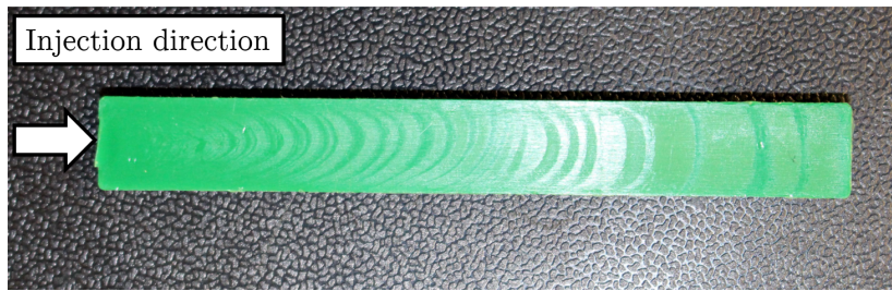
Figure 11 : Flow-induced material orientations in an injection molded rectangular bar of polypropylene
