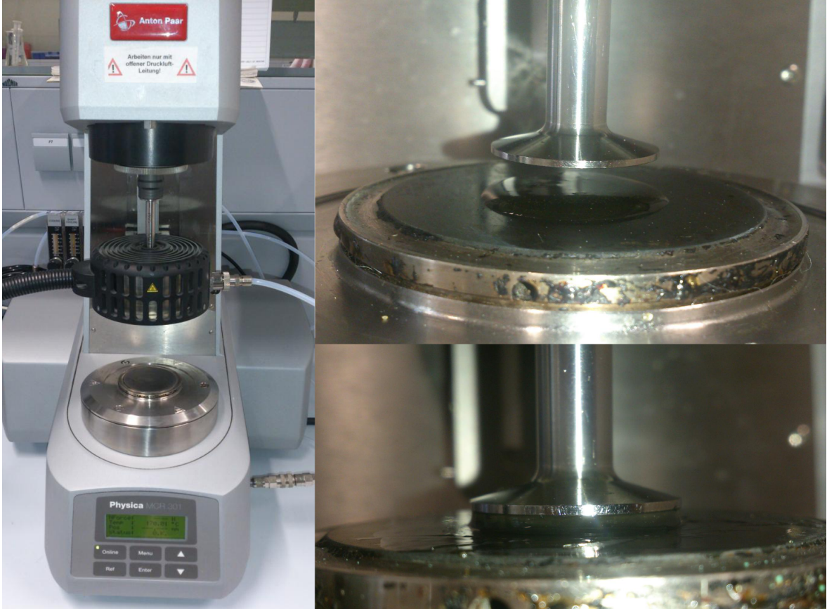
Figure 54 : Left: The used setup for the shear-rheological measurements. Anton Paar MCR 301 rheometer and a plate-plate measuring geometry with a diameter of 25mm (PP25) Top right: molten polymer specimen (prepared using VCM), before trimming, Bottom right: trimmed specimen, ready for measurement[47]
