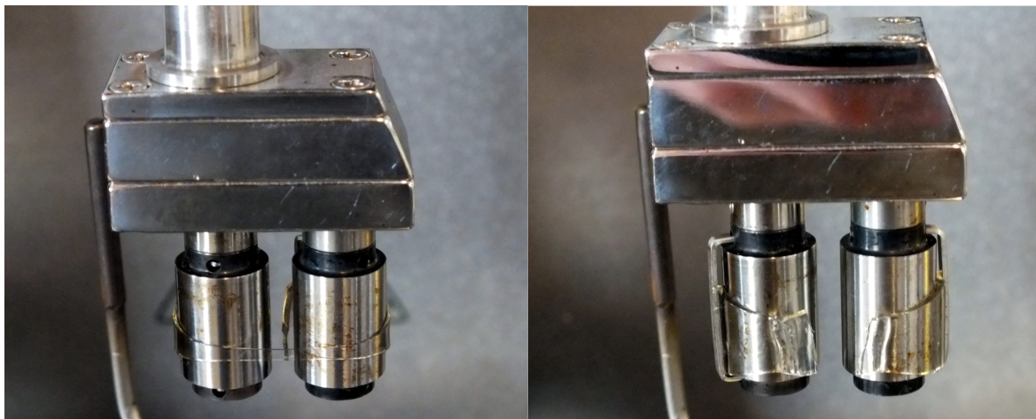
Figure 83 : Melt films of Soluplus ® after being stretched using the SER fixture at an extensional strain rate of 0.1s^{-1} (left) and 25s^{-1} (right)
