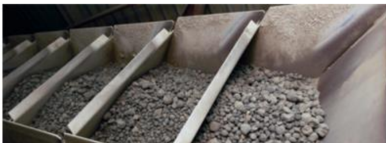
Figure 12: Loaded apron conveyor ( www.beumer.at )
