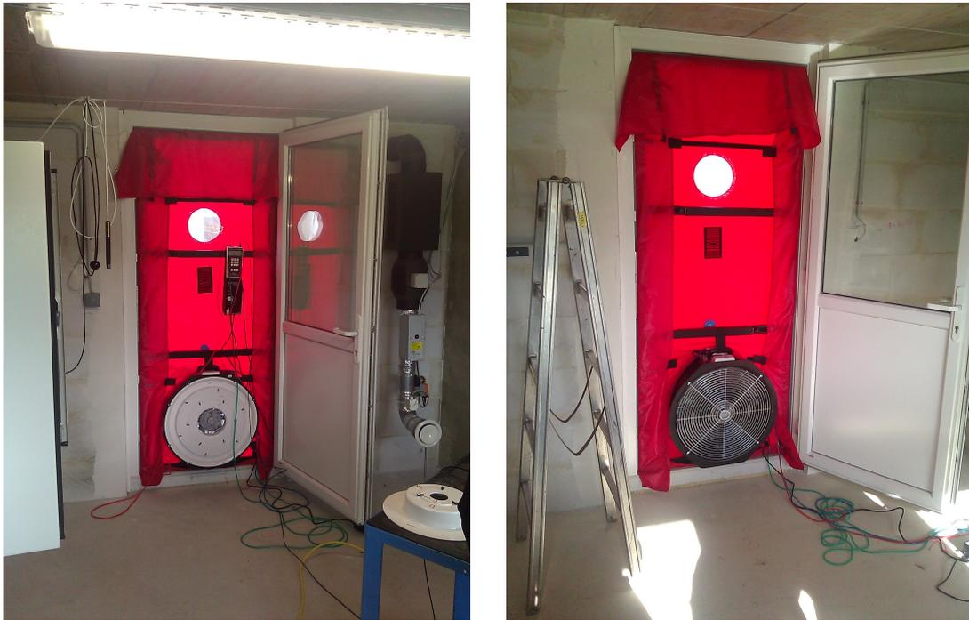
Figure D.7.: Blower door depressurization (left) and pressurization (right) test.
