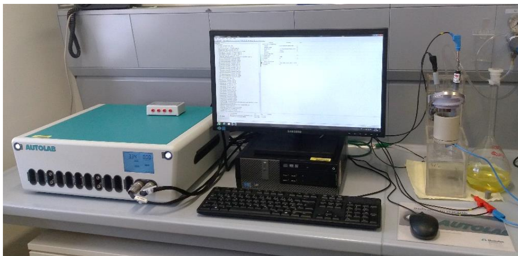
Figure 26: The measuring station with potentiostat on the left and electrochemical cell on the right
