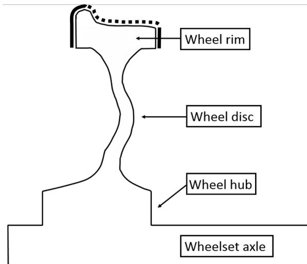
Figure 4.12: Three wheel areas for the convection cooling. The first area is the wheel tread (dashed line), the second is the side faces of the wheel rim (thick black lines) and the third is the surface of the wheel disc. [4]
