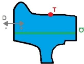
Figure 4.1: Railway wheel rim with three solutions: tread temperature  $T$ , residual stresses  $\sigma$  and wheel rim deformation  $D$
