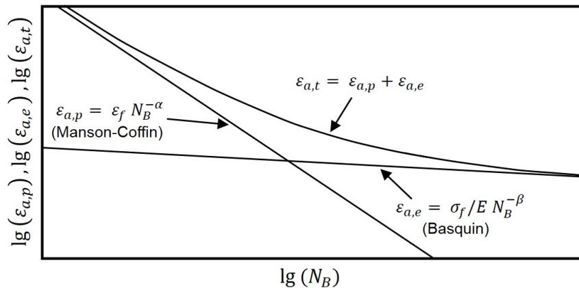
Figure 2.11: Schematic strain-Wöhler-curve with Manson-Coffin- and Basquin-relation [48]
