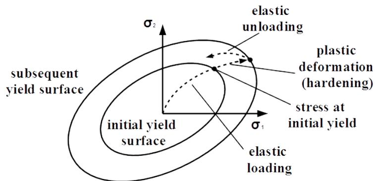
Figure 2.8: Yield surface of the isotropic hardening rule. [40]
