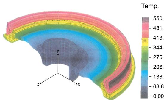
Figure 2.2: 3D FEM calculation of temperature distribution of a wheel sector [30]
