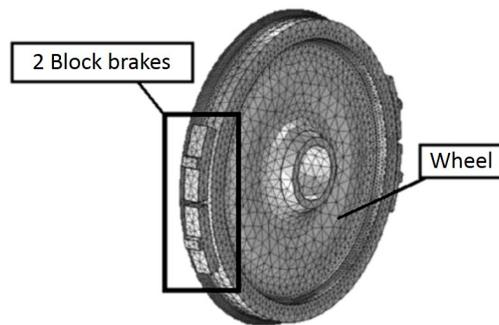
Figure 4.7: The three-dimensional model of the block-braked wheel. [17]
