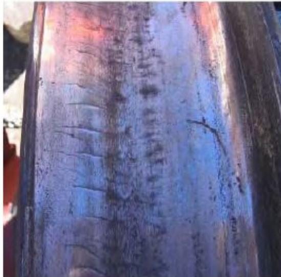
Figure 1.11: Rolling contact fatigue.
