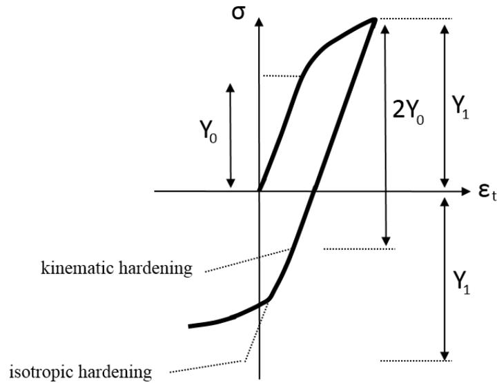
Figure 2.10: The Bauschinger effect: Comparison between isotropic and kinematic hardening [40]
