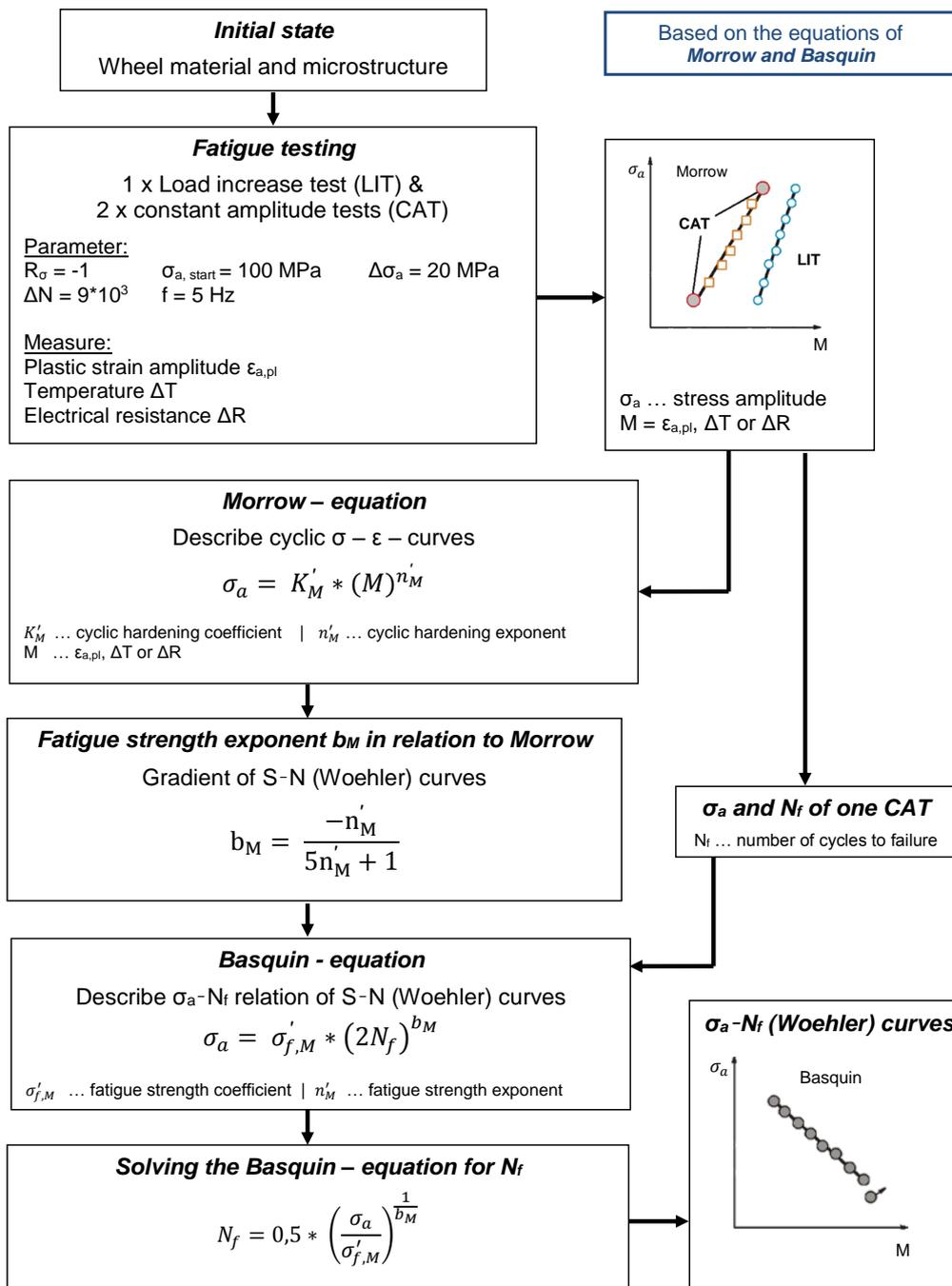
Figure 5.3: Lifetime calculation method based on the Basquin-model. [84] [85] [86] [87] [88].
