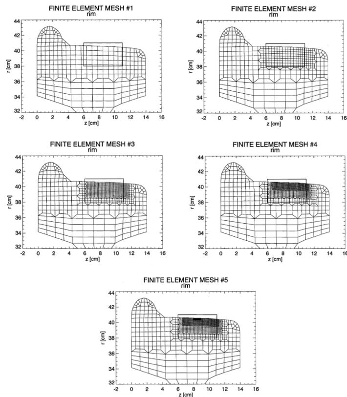
Figure 4.4: Different forms of meshes from the wheel tread. [60]
