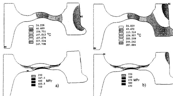
Figure 4.8: Temperature and stress states of the wheel with centred (a) and overhanging (b) block brake positions. [74]
