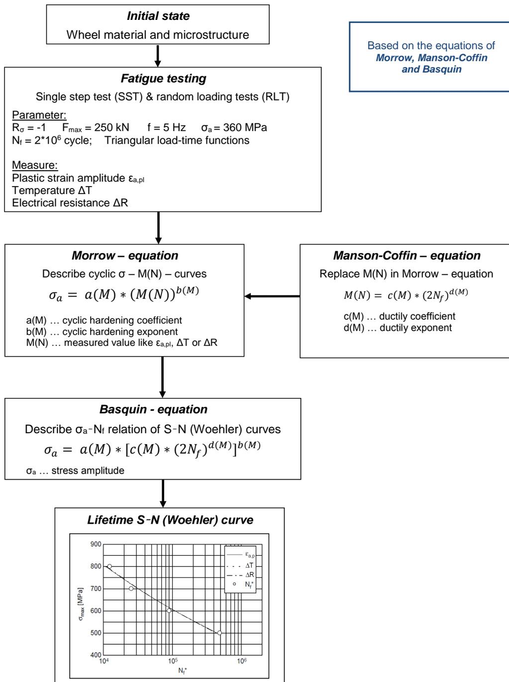
Figure 5.4: Lifetime calculation method based on the Basquin-Manson-Coffin-model. [89] [90] [91].
