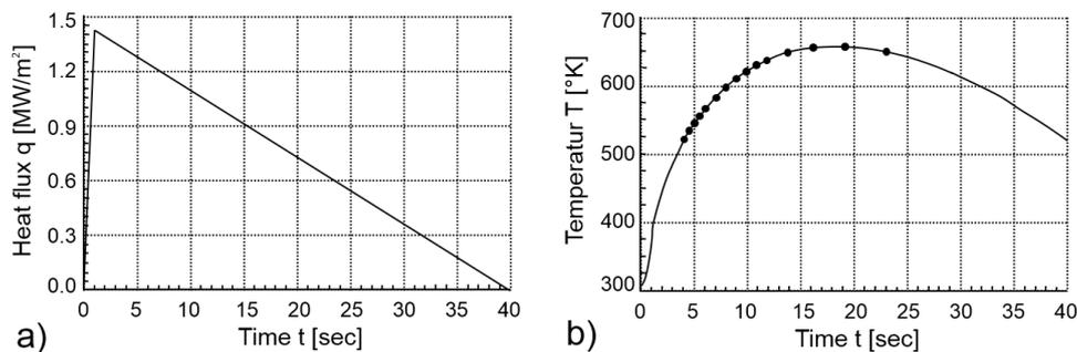
Figure 4.10: Heat flow-time curve (a) and temperature-time curve (b) on the wheel tread for one stop-braking. [60]
