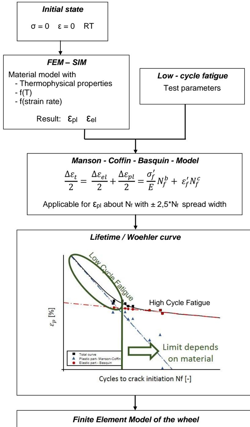
Figure 5.1: Damage model used by Siemens AG. [81] [82] [83]
