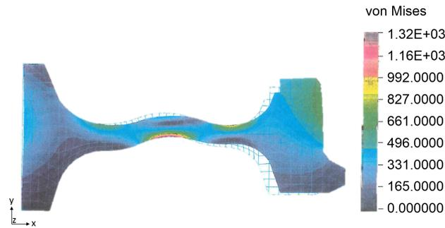
Figure 2.1: 2D FEM calculation of stress distribution and deformation of a wheel. [30]
