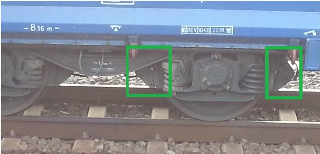
Figure 1.2: Freight trains with two brake blocks per wheel, indicated by the green boxes.
