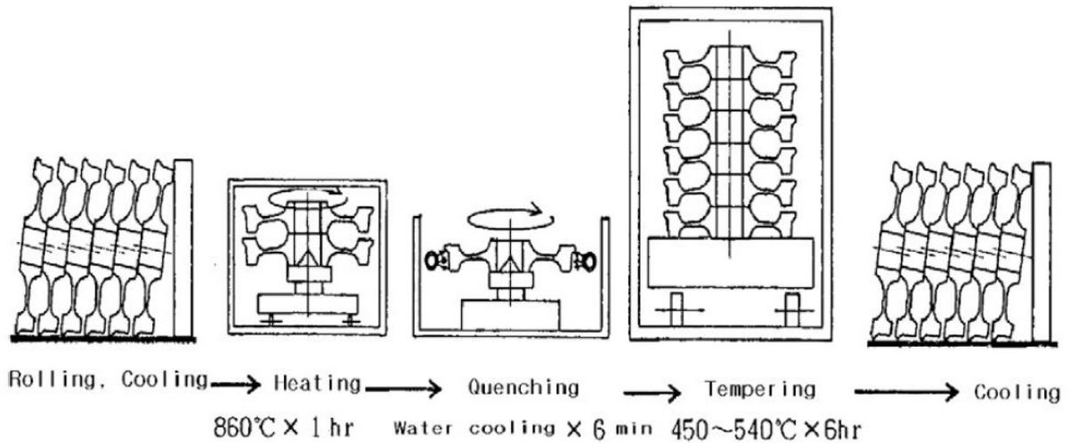
Figure 1.8: General illustration of a wheel heat treatment [15]
