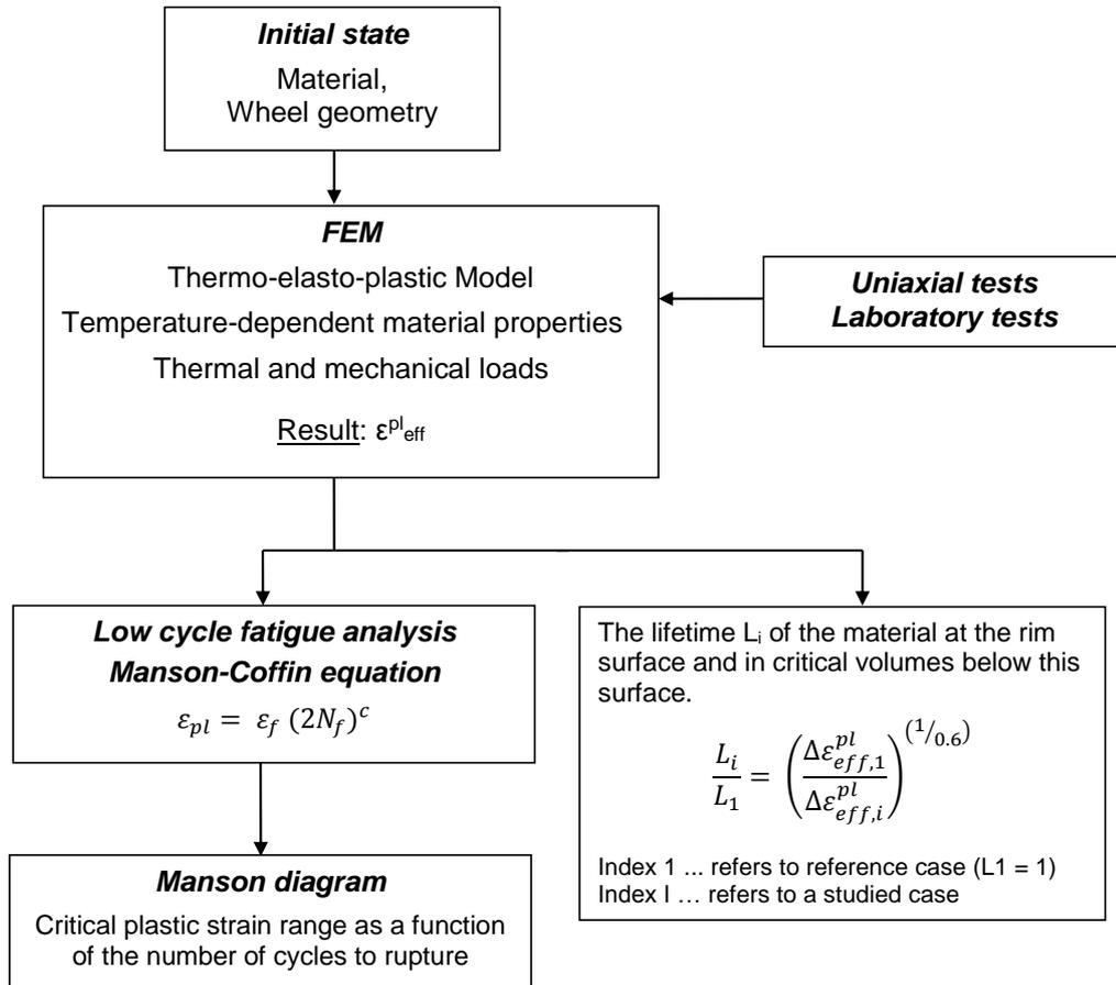
Figure 5.6: Lifetime measurement during thermo-mechanical load and based on Mason-Coffin-model [63].
