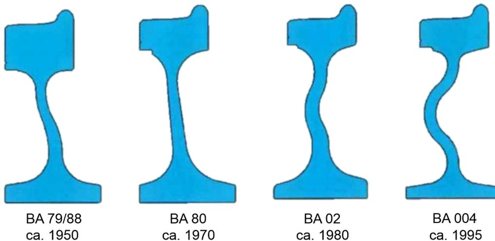
Figure 1.4: Development stages of block braked wheels [9]
