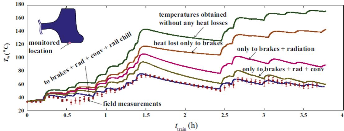
Figure 4.11: Different wheel rim temperatures received from finite element simulation. [18]
