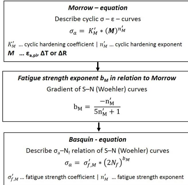
Figure 5.2: Relation between Morrow and Basquin-equation, which can be transformed into a general form, where  $M$  can be  $\Delta T$ ,  $\Delta R$  or  $\epsilon_{a,pl}$ . [84] [85].
