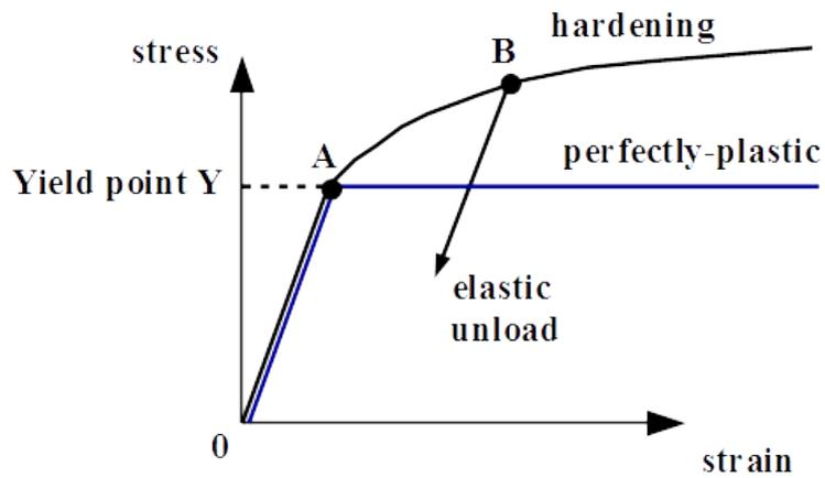
Figure 2.7: Uniaxiale strain-stress curve [40]
