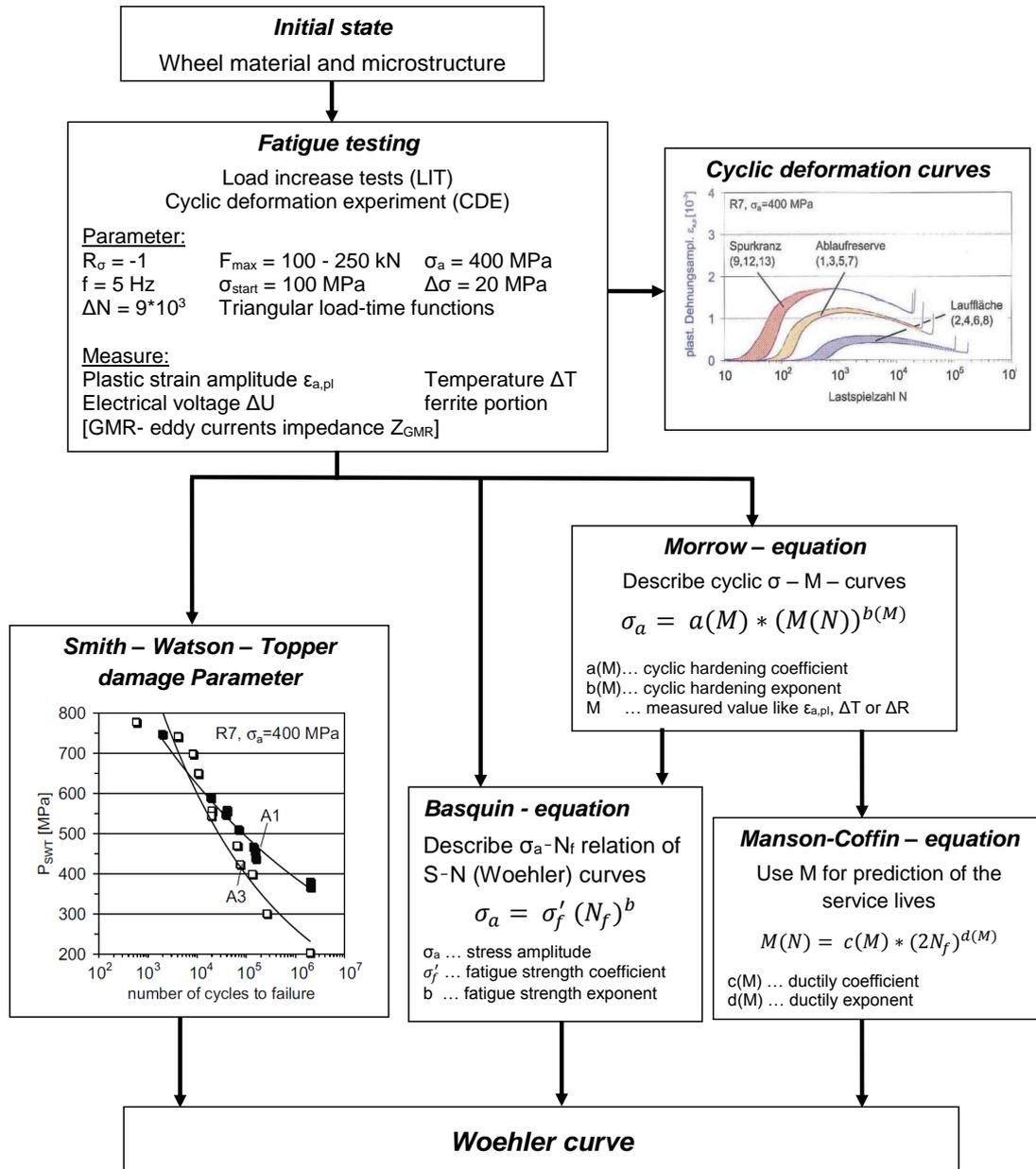
Figure 5.5: Lifetime calculation on the basis of Basquin-model, Manson-Coffin-model or Smith-Watson-Topper damage Parameter [13] [92] [93] [94].
