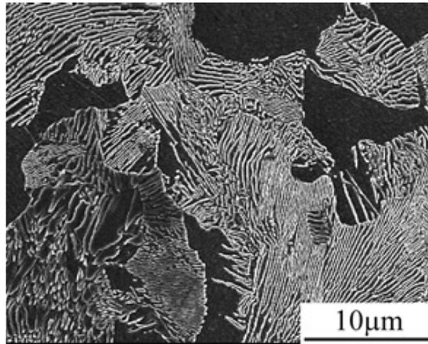
Figure 1.6: Characteristic microstructure close to the surface of the R7 monobloc wheel. [13]
