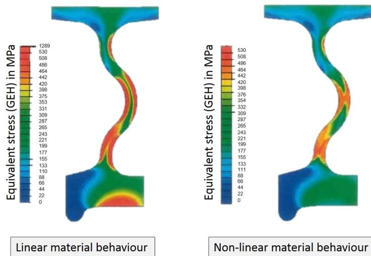
Figure 4.6: Comparison between the elastic and the elastic-plastic finite element models. [9]
