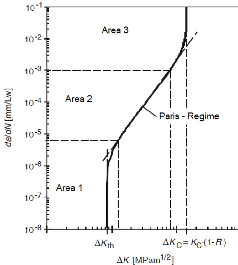
Figure 2.12: Crack growth curve [52]
