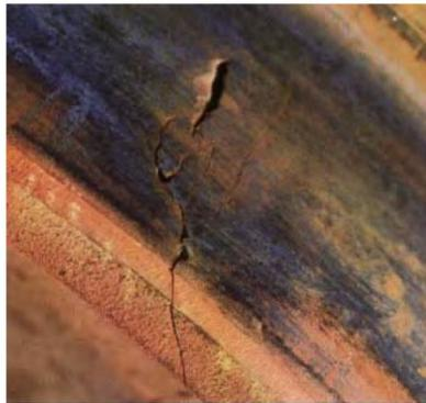
Figure 1.12: Fatigue crack originating from a thermal crack [19]
