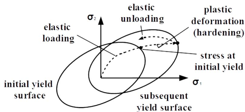
Figure 2.9: Yield surface of the kinematic hardening rule. [40]
