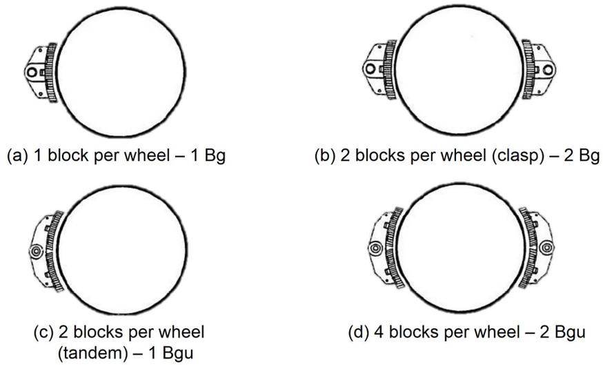
Figure 1.3: "Four common block arrangements. Two blocks can be used either in (b) clasp or (c) tandem arrangement. Bg and Bgu stands for "Bremsklotz geteilt" and "Bremsklotz geteilt unterteilt", respectively." [8]
