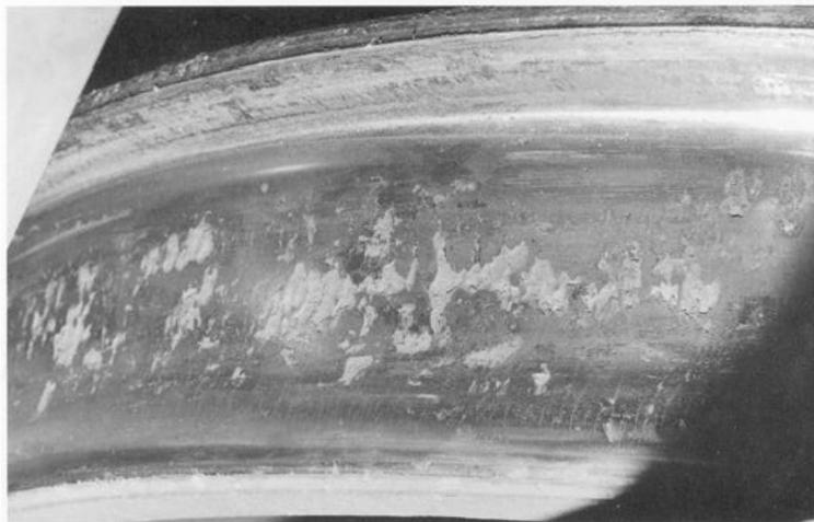
Figure 1.13: Spalling of the tread area [19]
