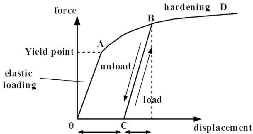
Figure 2.5: Force-displacement curve for metal at tension test. [40]
