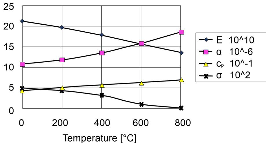
Figure 4.5: Material parameter as a function of temperature: Modulus of elasticity  $E$  [MPa], extension coefficient  $\alpha$  [1/°C], specific heat  $c_p$  [kJ/kgK] and yield stress  $\sigma$  [MPa]. [64]
