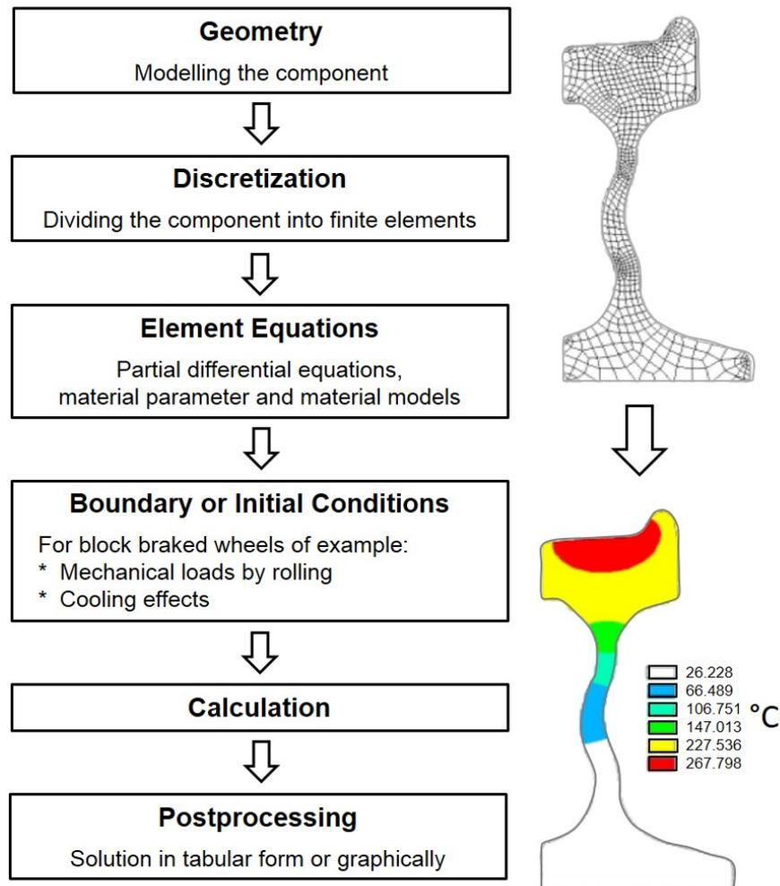
Figure 2.3: Finite element approach by a standard step-by-step procedure. At the bottom, part of the wheel is shown with finite elements and one possible solution for the temperature distribution. [30]
