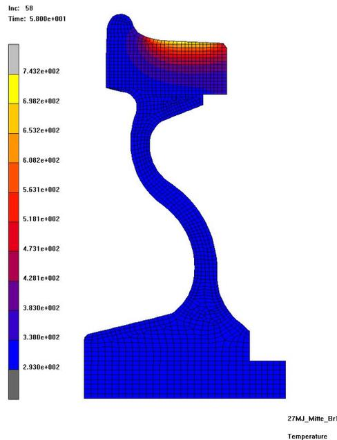
Figure 4.3: The graphical temperature result from the transient thermo-mechanical MARC model, [59]
