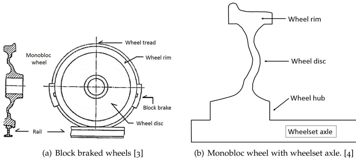
Figure 1.1: Block braked wheel system
