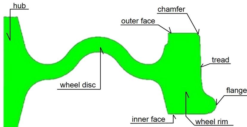
Figure 1.7: Cross section of a monobloc wheel
