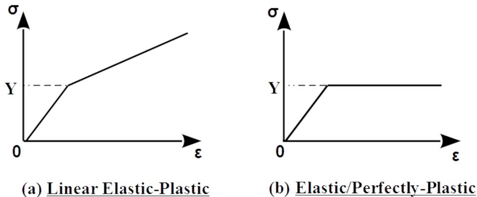
Figure 2.6: Comparison between (a) linear elastic-plastic and (b) elastic-perfectly plastic material model. Linear elastic-plastic include hardening above  $Y$ . [40]
