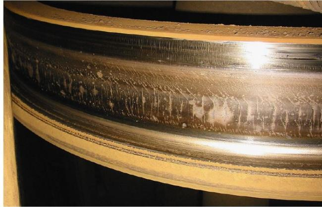
Figure 1.9: Tread thermal cracking in an actual railway wheel. [24]
