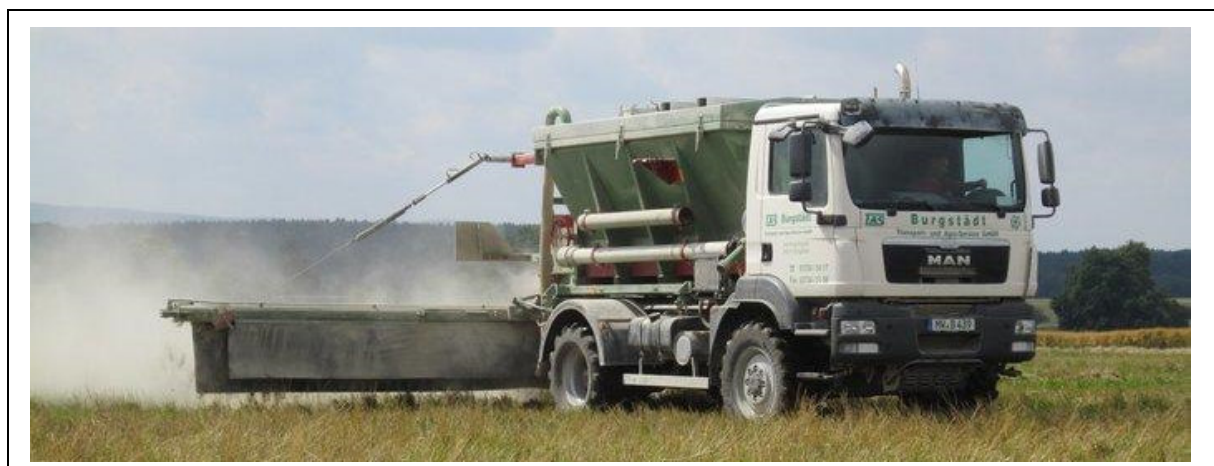
Figure 42: Lime sand spreader mounted on truck 196
