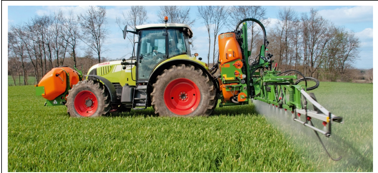
Figure 37: Mounted crop sprayer behind standard tractor with additional tank in the front 191
