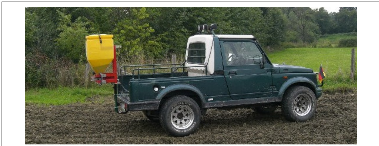
Figure 40: Small disc spreader mounted on compact SUV 195
