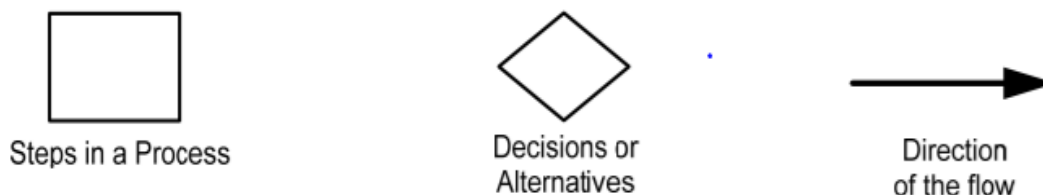
Figure 14: Common symbols used for creating flowchart [30]
