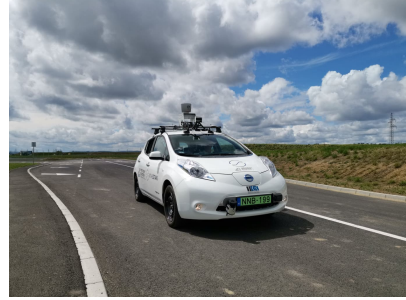
Figure 1. Electronically modified autonomous test vehicle
