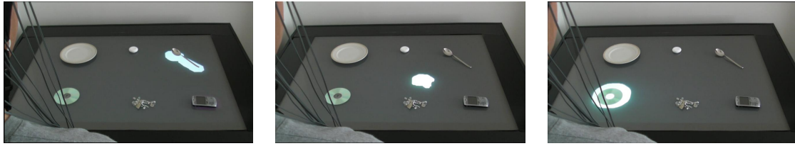
Figure 2: A participant interacting with the multi-touch table P300-based BCI from [7]. Six objects have been placed on the table. Left: The spoon is flashed by surrounding it with light. Centre: A non-object flash. Right: The area around the CD is being flashed.
