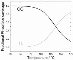
Fig.6. Adsorption of  $H_2$  and CO on platinum as a function of the temperature. Adopted from [5].
