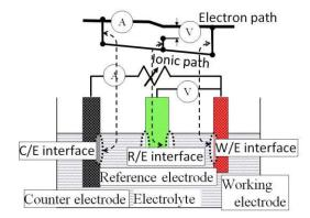
Fig. 1 Schematic drawing of 3-electrode electrochemical cell with their potential profile image.
