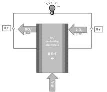
Fig.4. Non-membrane based mixed electrolyte
