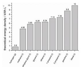
Fig.1. Energy density of various liquid fuels.
