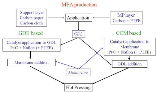
Figure 6: Resuming scheme of MEA preparation process.
