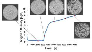
Fig. 3: Simultaneous measurements of oxygen diffusivity and water visualization by X-ray CT
