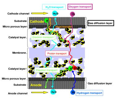
Fig.2: Mass transport factors around cathode catalyst layer
