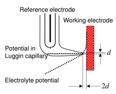
Fig. 2 Schematic drawing of the Luggin capillary.
