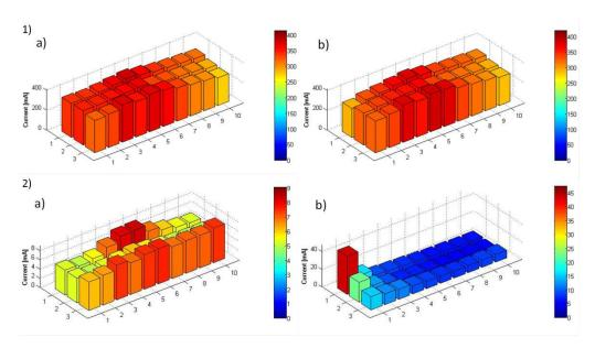
Fig. 3: Current distribution 1) at 400 mA/cm² and 2) hydrogen diffusion measurement at 430 mV for a) a pristine MEA and b) a MEA perforated at segment 1.
