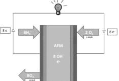
Fig.3. Anion exchange membrane (AEM) based DBFC.
