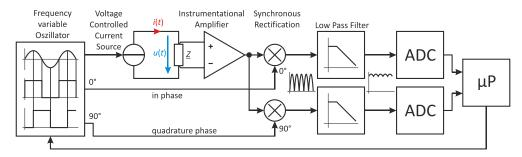
Figure 5: Signal generator, VCCS, quadrature synchronous rectification, A/D converters
