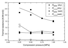
Fig. 4: Thermal resistance of GDL and its boundary
