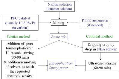
Figure 5: Resuming scheme of catalyst layer preparation procedure.
