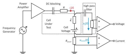
Figure 4: Impedance measurement, taking account of cell voltage
