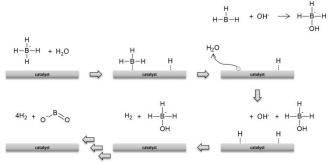
Fig.2. Proposed mechanism of catalytic borohydride hydrolysis.
