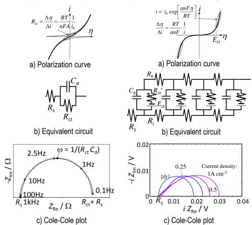
Fig. 10 Typical electrochemical AC impedance spectroscopy for fast reaction.
