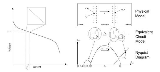
Figure 1: Fuel Cell Voltage / Current and Impedance Characteristic
