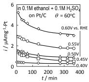
Fig. 8 Chronoamperogram of Pt/C for ethanol oxidation reaction.
