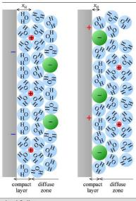
Figure 13.4 Cartoon of the supposed structure of the interfacial region of a double layer when the electronic conductor is charged negatively (left) or positively (right). Only a small portion of the diffuse zone is shown.
