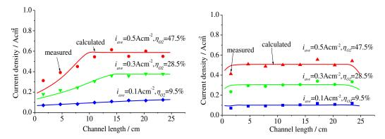
Fig. 5: Measured and calculated current distributions (left: co-flow, right: couter flow)
