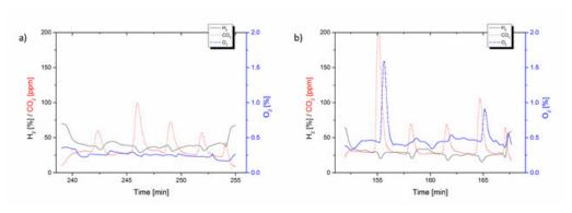
Fig. 6: Anode off-gas analysis of a) a pristine MEA and b) a MEA perforated five times.
