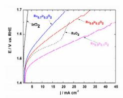
Linear polarization of different Ru-based anode catalysts in 0.5 M  $\rm H_2SO_4$  at 5 mV s<sup>-1</sup> and 20 °C. (half cell).
