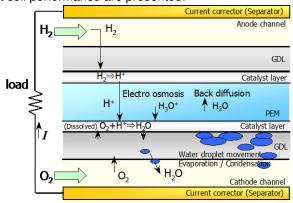
Fig.1: General factors of water transport inside PEFC
