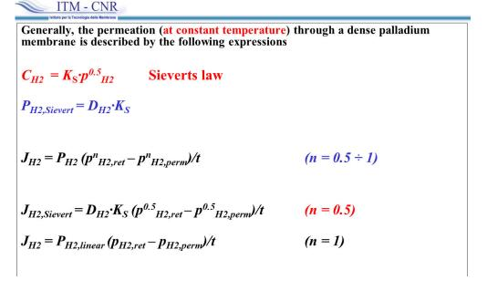
Figure 4. Equation relating the hydrogen transport in Pd-based membranes
