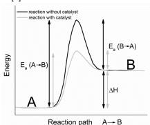
Fig.5. Activation energy of a reaction.
