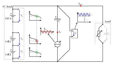
Typical Distortion Analysis Measurement Setup (also suitable for EIS)
