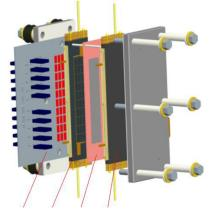
Fig. 2: Design of a 25 cm² segmented fuel cell: 1) current collector with resistors, 2) segmented cathode plate, 3) MEA, 4) anode plate.
