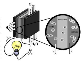
Fig. 1: Principle of a PEFC.
