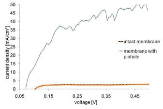
Fig1: Hydrogen diffusion current measurements
