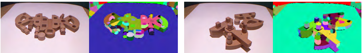
Figure 3: Point cloud segmentation generated by a color-based model-free method.
