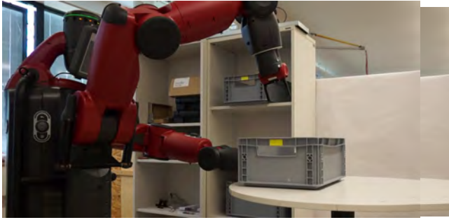
(a) Baxter inspecting the box with its end effector camera.
