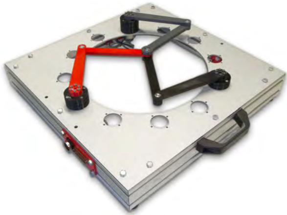
Figure 1. Platform with three arms (motor, active link, passive link) in different colors
