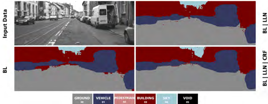
Figure 3. Improvement of segmentation quality of background classes (BL: baseline method, LLN: Local Label Neighborhood, CRF: Conditional Random Field).
