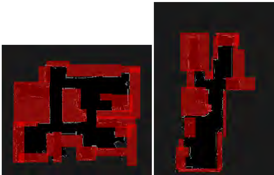
Figure 5. MIRA no-go areas can be added in order to avoid undesired global paths when the static map is cleared. In very narrow corridors, however, some margin must be left to account for possible localization errors.
